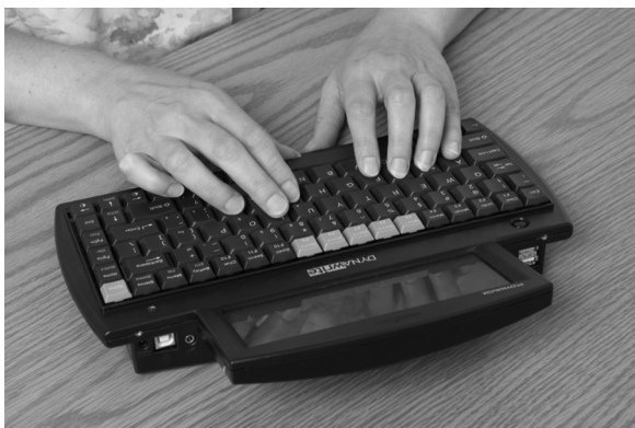
Fig. 20.3. A portable key-board-activated communication device with voice output. The device is lightweight and is powered by a rechargeable battery.
