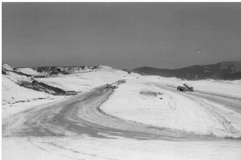
Fig. 23.2. Mining operations of the Lompoc Diatomite, an upper Miocene marine diatomite. Excavation and transport vehicles are more than 6 meters high. (Photo by E. F. Stoermer.)
