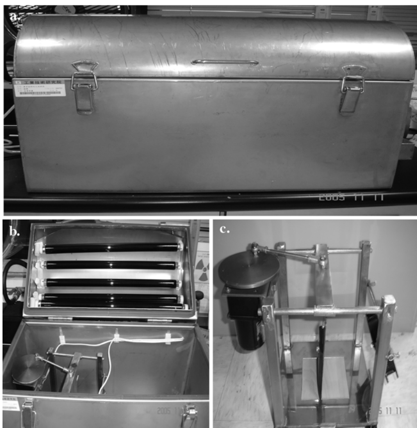
Figure 1. The simulation box. (a) appearance, (b) inner, and (c) the fan, rubber knife and substrate.
