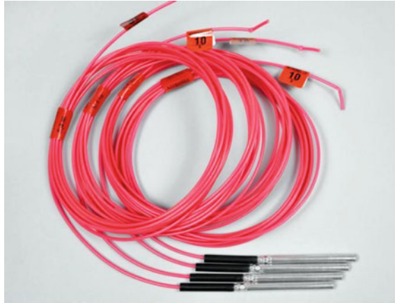
Fig. 4.14 Shock tube detonators (Nonel)
