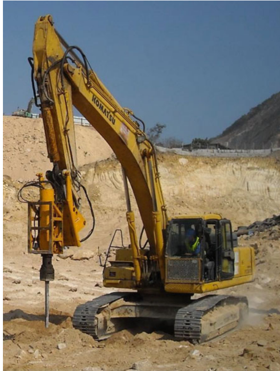
Fig. 7.7 Excavator-mounted hydraulic splitter
