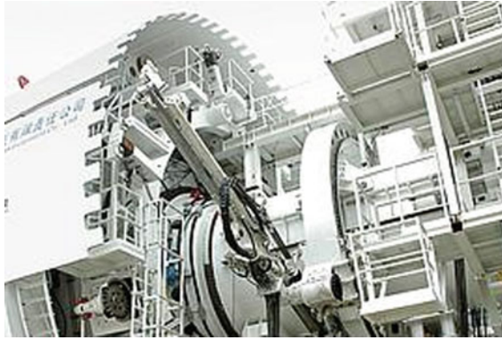
Fig. 14.27 The rock support anchors have to be installed by the roof bolting systems directly behind the shield. (Source www.herrenknecht.com/ )
