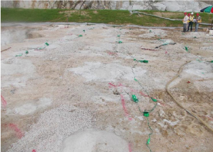
Fig. 8.21 Bench surface after completion of firing connection with SmartShot electronic detonators in KWP Quarry, 2013
