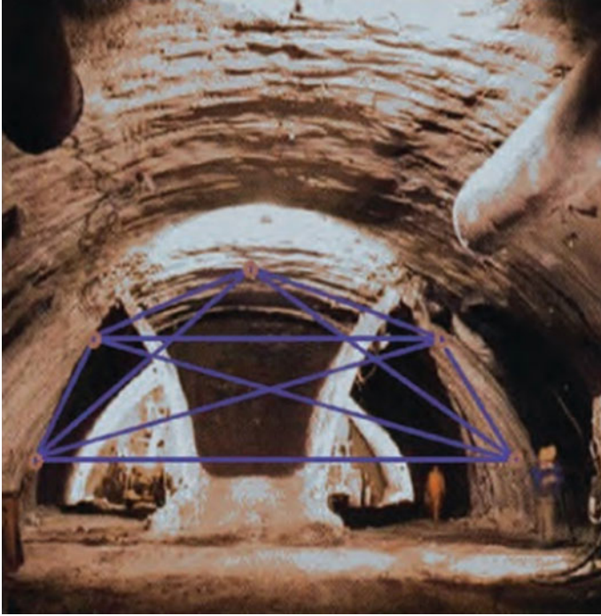
Fig. 22.21 Illustration of optical 3D convergence measurement, measurement results are absolute, accuracy 1–2 mm for monitoring the deformation of cavity deformation of the tunnel walls surface (reproduced from Ref. [2] with the permission from AITES/ITA)
