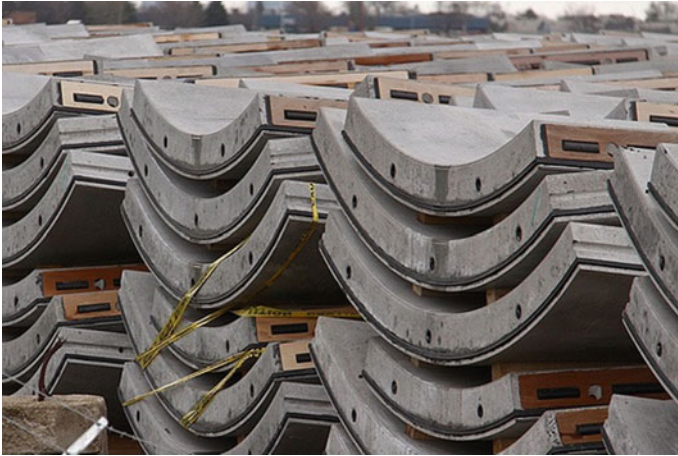
Fig. 21.45 Precast concrete segment for tunnel support
