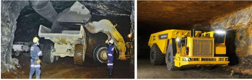
Fig. 19.2 Wheel loader and dump truck combination ( left ) and Minetruck MT 5020 ( right ) (Reproduced by permission of Atlas Copco)
