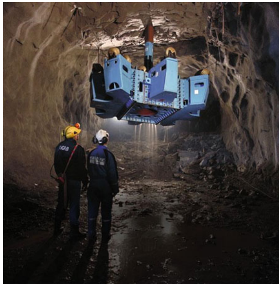
Fig. 14.9 A reamer is raising for reaming (Reproduced from Ref. [3] by permission of Sandvik)
