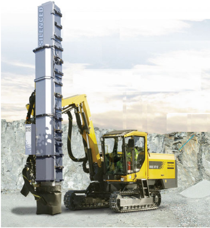
Fig. 2.31 Silenced drilling rig (Reproduced with the permission from Atlas Copco)
