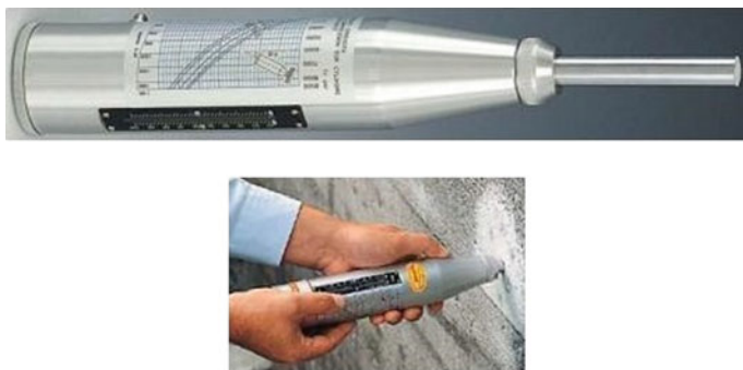
Fig. 1.7 Schmidt Hammer rebound hardness test (Source [10])
