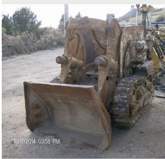
Fig. 19.17 Eimco 630 air mucking machine (Source www.savonaequipment.com/en )
