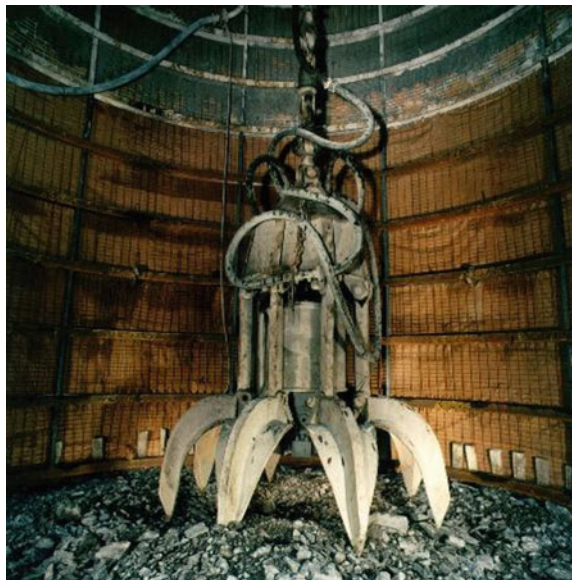
Fig. 19.16 Cactus grab manufactured by DH Mining Systems (Source www.dhms.com.en )
