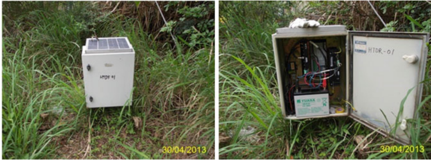
Fig. 22.22 Time-domain reflectometer probe for detecting slope movement
