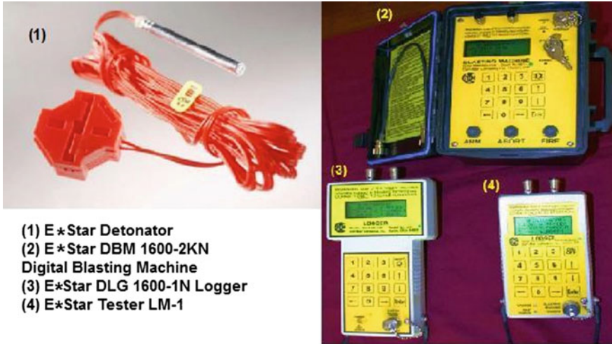
Fig. 4.27 Austin E*Star electronic blasting system. 1 E*Star detonator. 2 E*Star DBM 1600-2KN digital blasting machine. 3 E*Star DLG 1600-1N logger. 4 E*Star tester LM-1
