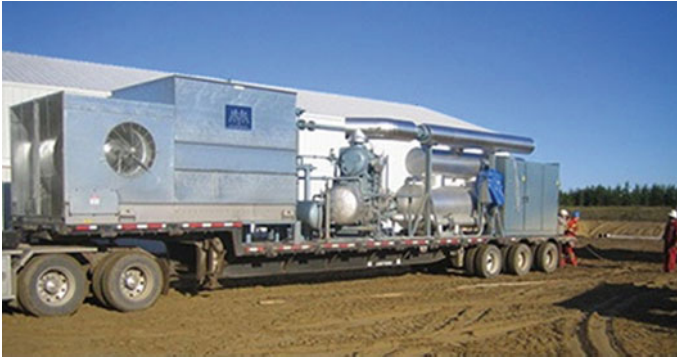
Fig. 21.7 Movable refrigeration unit Source www.mmrefrigeration.com
