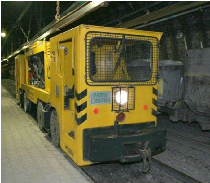
Fig. 19.11 Electric locomotive for tunnel transportation
