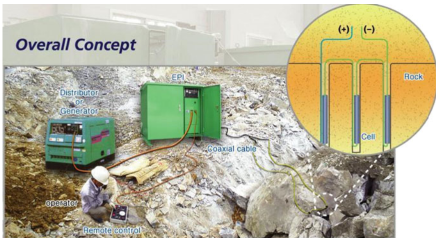
Fig. 7.16 Overall of pulse plasma rock fragmentation technology (Source Kapra & Associates, Korea)
