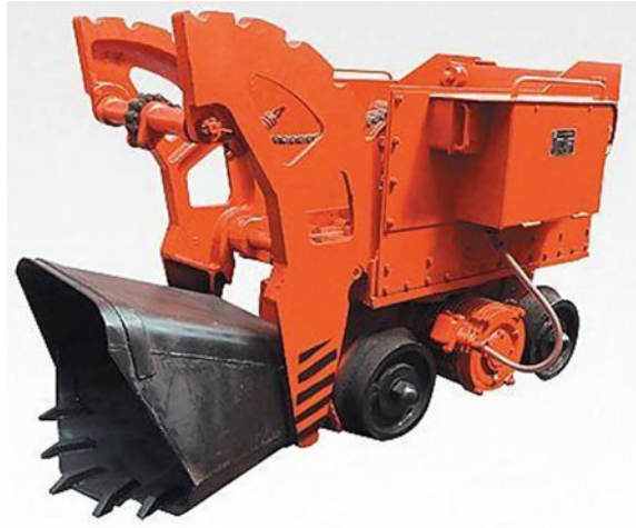
Fig. 19.1 Overhead shovel loader, rail-mounted
