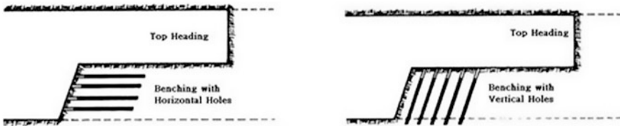
(c) Bench blasting with Horizontal or vertical drill holes
