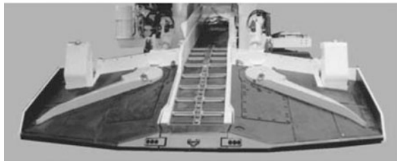
3 Two lateral loading beams
