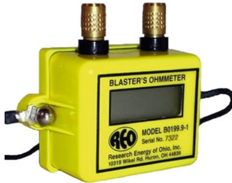
Fig. 4.9 Ohmmeter for measuring the resistance of electric detonators
