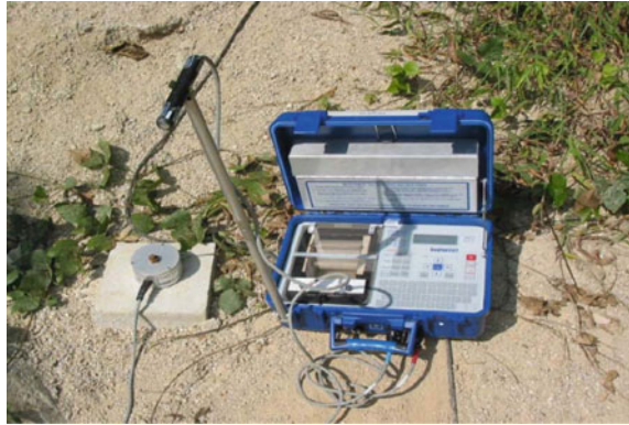
Fig. 6.7 Vibration and air overpressure monitoring
