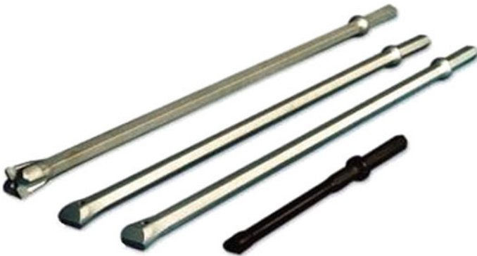
Fig. 2.40 Integral drill steels
