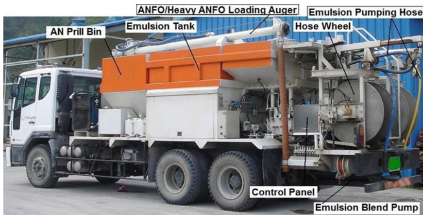
Fig. 3.46 Multi-function mobile manufacture unit (MMU)
