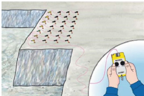
Fig. 4.21 Firing a blasting round using a blasting machine (Dyne Nobel)
