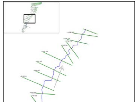
Figure 7. Geometric data generating from Hec-RAS.
