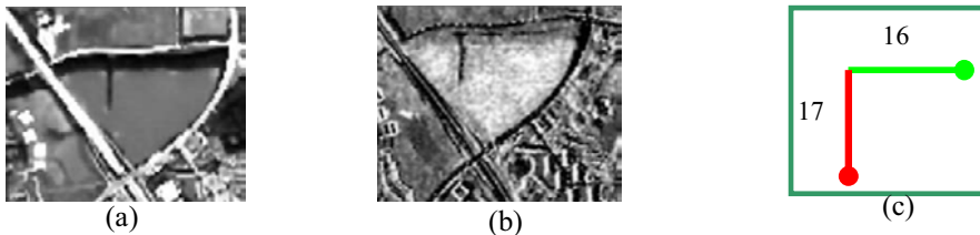
Figure 4: Test region of the optical image (a), Test region of the SAR image (b), Real translations between images in pixels (c)
