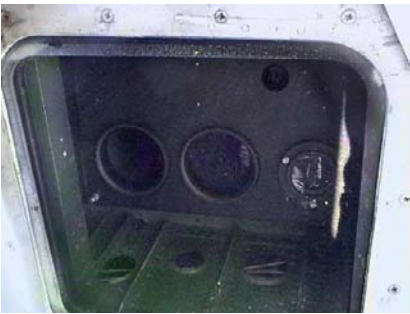
Figure 3. Optical LIDAR unit in photo-camera hatch.
