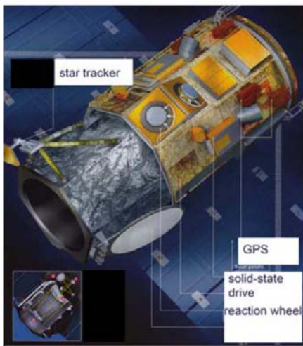
Figure 2. GeoEye-1; Typical hardware components of a high resolution optical satellite courtesy: GeoEye.
