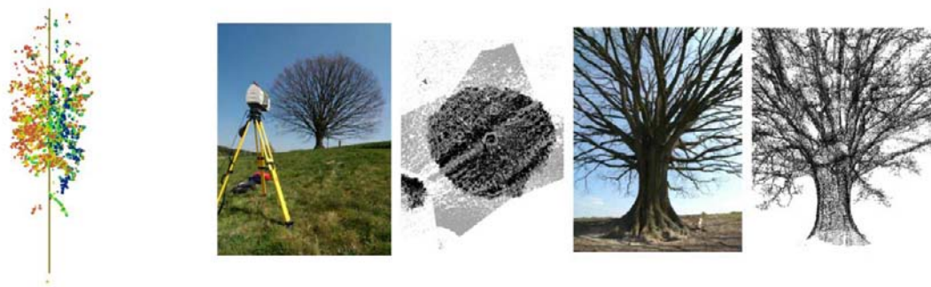
Fig 3. Voxel model of Picea abies (left), photographs and results of Quercus petraea scanning (position, crown in a horizontal level, tree photo, result of the scanning)
