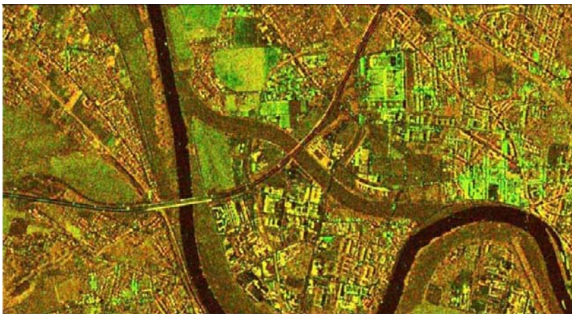
Figure 6. Multi polarization (HH/VV) TerraSar-X SpotLight image reduced by factor 2 city of Dresden.
