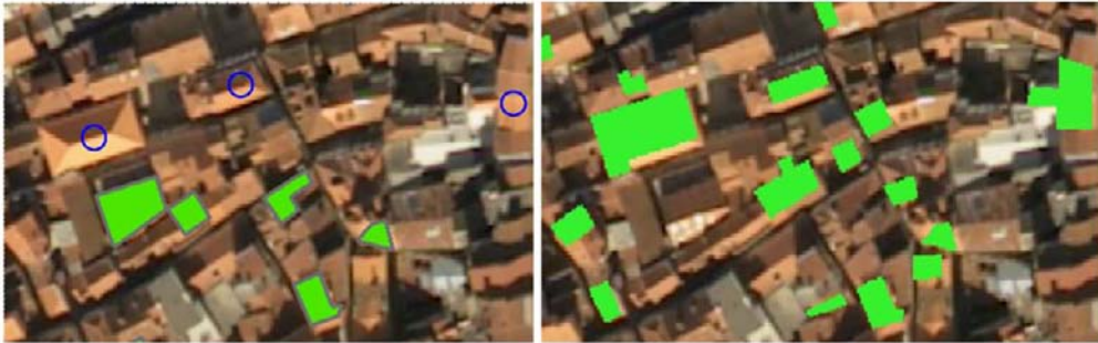
Figure 8. a) Extract of the aerial image (RGB321) overlaid with the buildings with ceramic tile roof not deteriorated classified by the University of Coimbra using traditional methods. b) Extract of the aerial image (RGB321) overlaid with the buildings with ceramic tile roof not deteriorated classified by the new approach. The circles mark some of the buildings which roofs were repaired or replaced by new ones and were correctly identified with the new classification approach.
