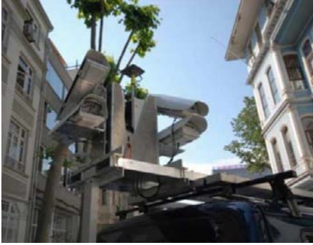
Figure 4. Intergrated GPS, INS, TLS and video camera components of a mobile TLS.
