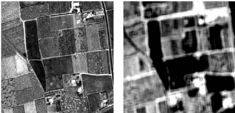
Figure 3: Panchromatic image (left) and Entropy index (right) of a subset of the studied image.
