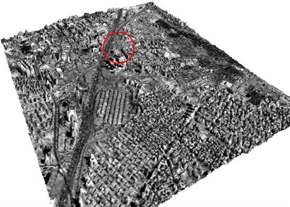
Figure 4. Part of drupe created out of along-track stereopair. Due to big image displacement of the buildings shown in Fig. 2, mismatches lead to errors in the DSM. From a theoretical point of view, redundant information from a third image could reduce this error.
