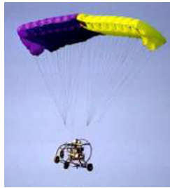
Fig. 2.3 An unmanned powered paraglider (Thamm and Judex 2006)
