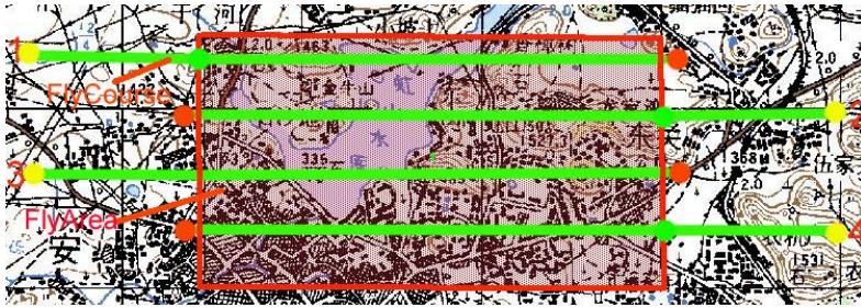
Fig. 2.13 The air route designed for remotes sensing experimental flight of the unmanned aircraft in Anshun, Guizhou Province in 2005
