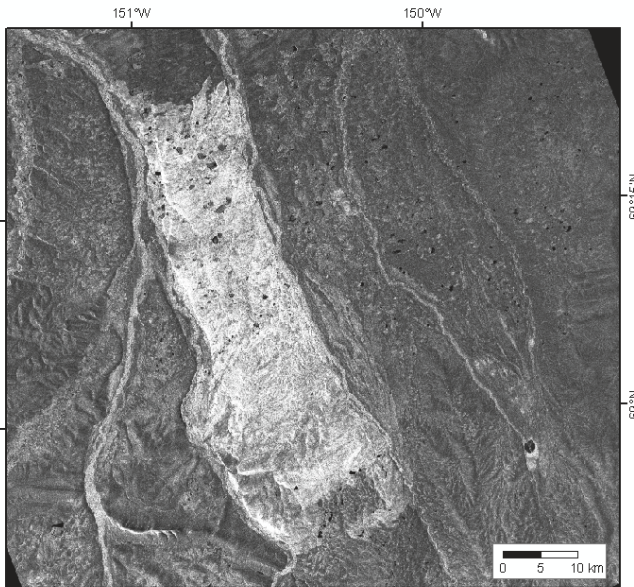
Fig. 7.6 Burn scars of the Anaktuvuk River Fire from July 2007, captured by an ERS-2 SAR image. The re-vegetated burned area shows a significantly higher backscatter than the surrounding areas assisting delineation of fire affected areas. Image © European Space Agency, 2008.
