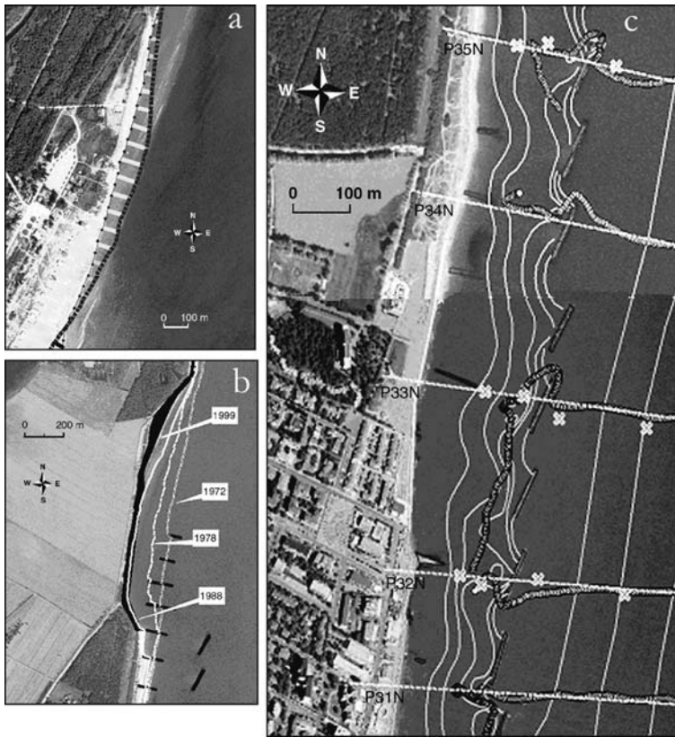
Fig. 33.2 Detail of coastline evolution: (a) changes between two successive coastline traces: 1972 ( black points ) and 1978 ( points and line ) are measured on crosswise transects that show distance values ; (b) beaches retreating (from 1978 to 1999) in concomitance with groins built before 1936 (the five northern groins were demolished during 2000). In black , a near shore seawall, built during 1999; (c) nearshore isobaths ( light grey lines ), samples location ( crosses ) and sedimentological profiles ( dashed lines ) done during the main Volano Project and included in the geodatabase
