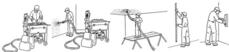
Fig. 3.18 Execution and spraying procedure of nontraditional gypsum plasters [26]
