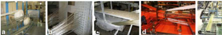
Fig. 11.8 Different stages of the pultrusion process: (a) creel and mat racks for fibre handling, (b) orifice plate, (c) open bath (courtesy of ALTO), (d) preforming guides, (e) cutting system (courtesy of Strongwell)
