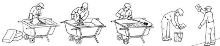
Fig. 3.17 Manual execution procedure of nontraditional gypsum plasters [26]
