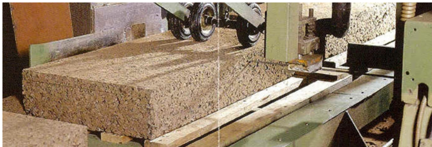
Fig. 13.7 Cutting the block into boards
