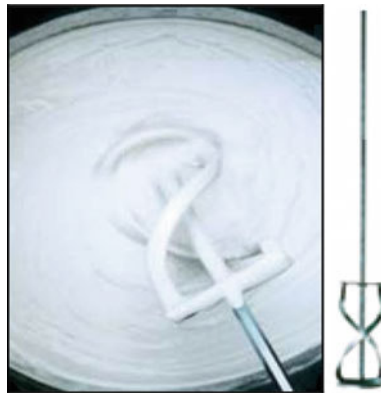
Fig. 3.44 Mixing with a double spiral mixer [31]
