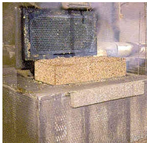
Fig. 13.6 Block of expanded agglomerated cork, coming out of the autoclave
