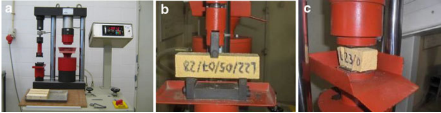
Fig. 2.8 (a) Strength test equipment [30]; (b) flexural strength test; (c) compressive strength test
