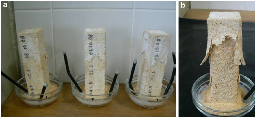
Fig. 2.15 (a) Test by contamination of mortars by capillary rise of a solution of sodium chloride at 15 %; (b) sample at the end of the test [photos by R. Nogueira]
