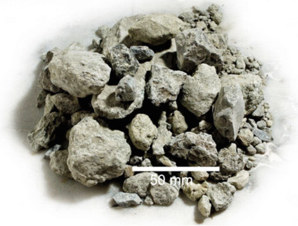
Fig. 1.8 Gypsum at clinker mill inlet
