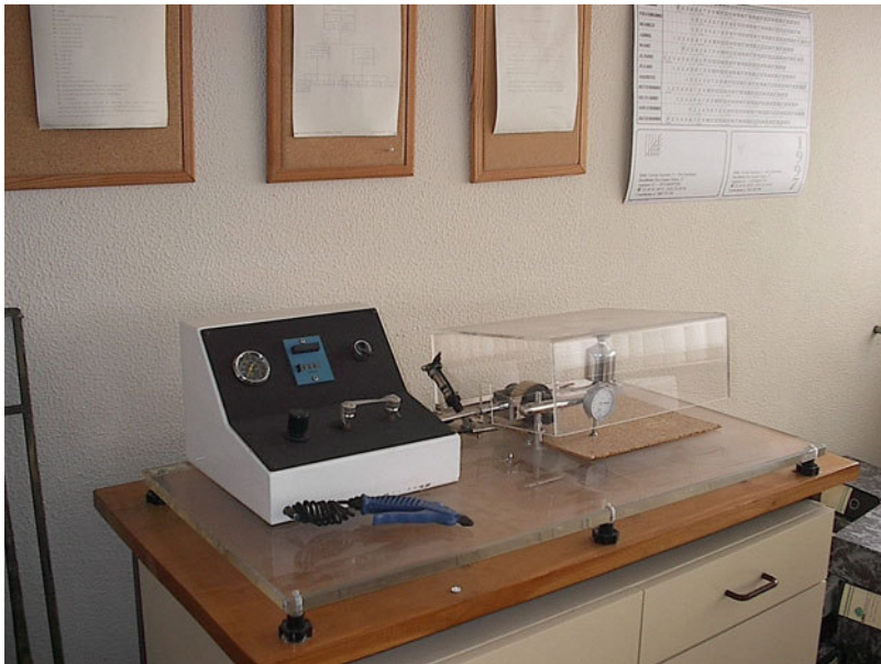
Fig. 13.15 Abrasion test for cork flooring
