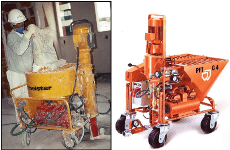
Fig. 3.46 Mixing with the spraying device itself [39, 40]
