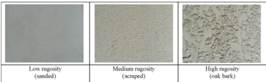
Fig. 2.29 Rugosity of premixed mortar coatings [42]
