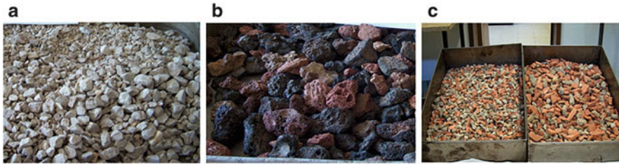
Fig. 20.8 Aggregates samples: (a) limestone natural aggregate; (b) non-crushed natural aggregate—Azores “bagacina”; (c) recycled aggregate
