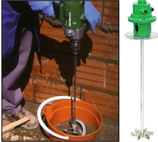
Fig. 3.45 Mixing with an electric mixer [35, 38]
