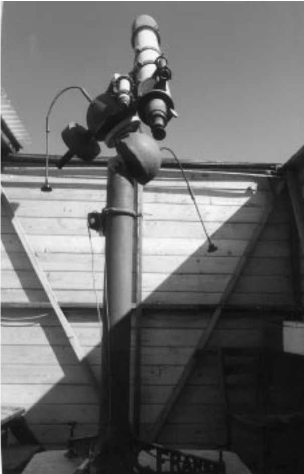
Figure 15.6 The 5-in refractor housed in the run-off roof shed.
