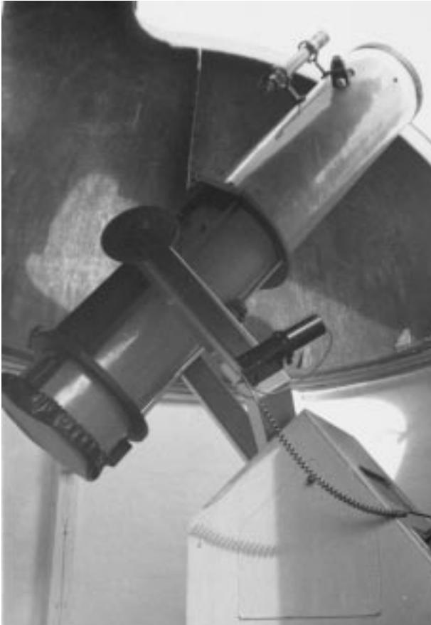
Figure 23.3 The 320 mm Newtonian on its fork mount.
