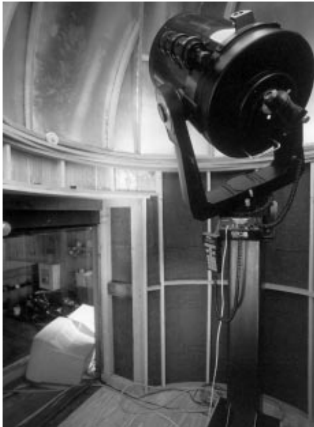
Figure 6.4 The Meade 300 mm SCT under the 1.7 m dome is computer-controlled from behind the observation panel in the main observatory.
