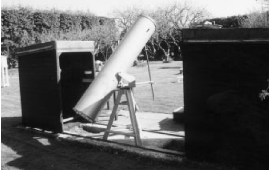
Figure 15.9 (above) The two-part run-off shed provides an unhindered view of the sky.
