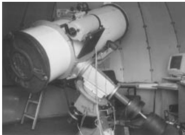
Figure 17.2 The 500 mm Newtonian telescope, with 150 mm Schmidt-Cassegrain guide scope.
