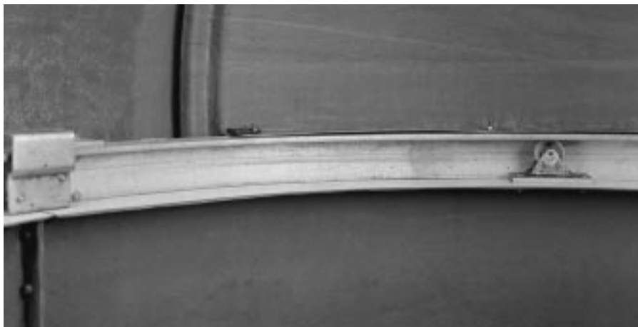
Figure 18.4 The L-shaped aluminium ring and one of the three rollers it rests on.
