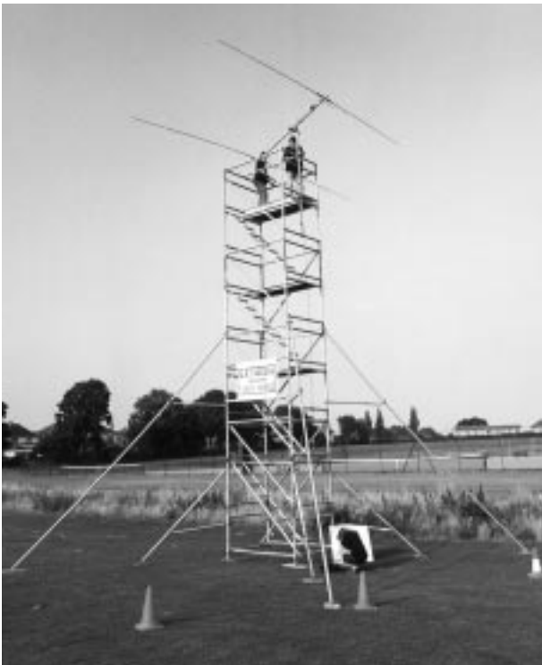
Figure 8.6 One of the two scaffold towers built to observe Jupiter's radio waves.
