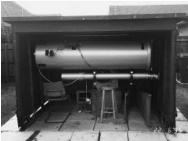
Figure 20.3 Eastern doors opened to show the 0.49 m (19 in) f/4.5 Newtonian in the stowed position.
