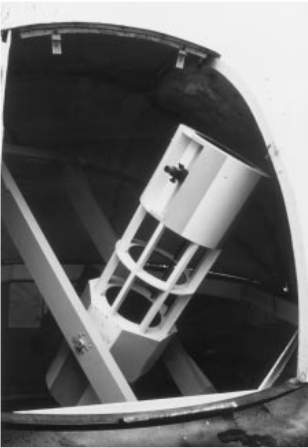
Figure 11.7 The 297 mm (11.7 in) and the English mounting, viewed through the open dome. Note the base-ring of the dome at the bottom of the photograph.
