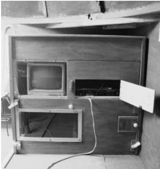
Figure 2.4 The CCD and computer cabinet under one of the observatory's corners.
