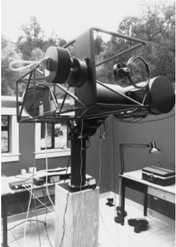
Figure 21.2 The ArchImage mount holding the 12½ in Newtonian and 11 in Schmidt-Cassegrain.
