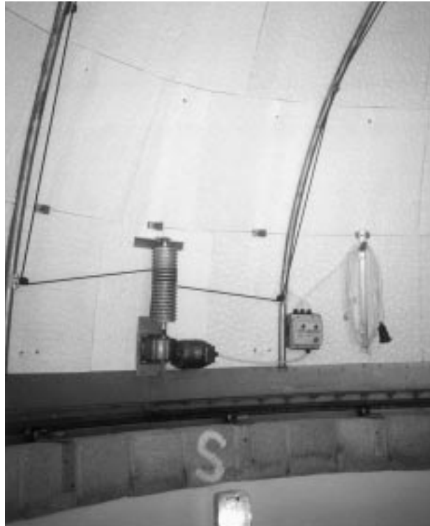
Figure 14.3 The “worm” which operates the ropes to open and close the dome slit.
