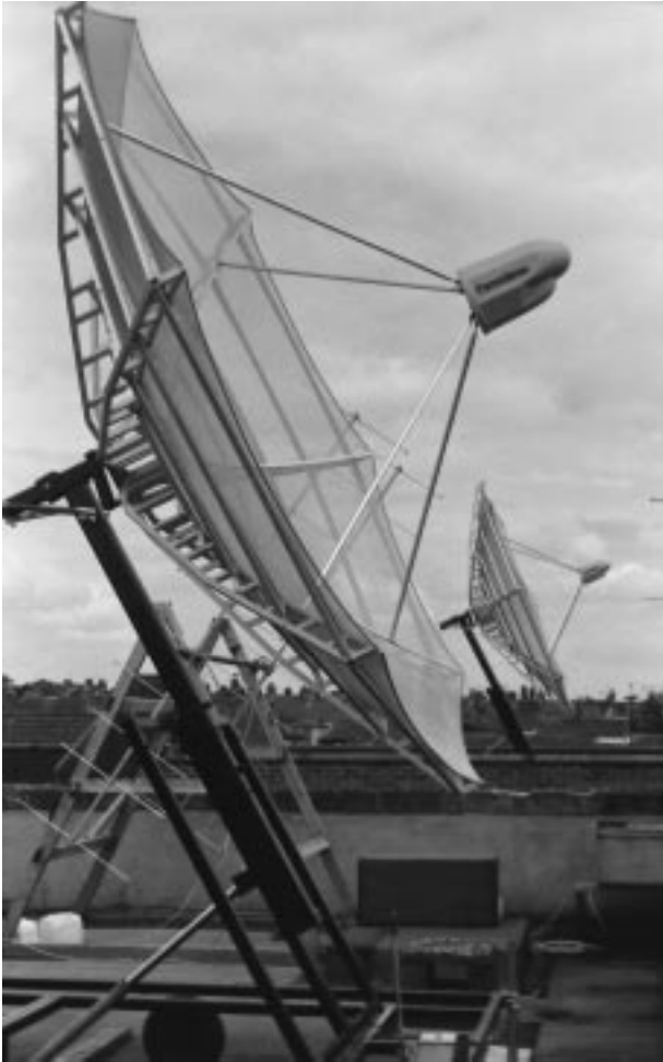
Figure 8.1 Satellite dishes to pick up microwaves at 1420 MHz, and the aerials used for the solar flare detector at 150 MHz. They are photographed on top of the school science block roof.
