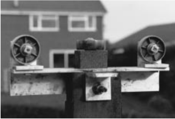
Figure 23.7 The wheel assembly: three wheels mounted on a pivoted aluminium angle.
