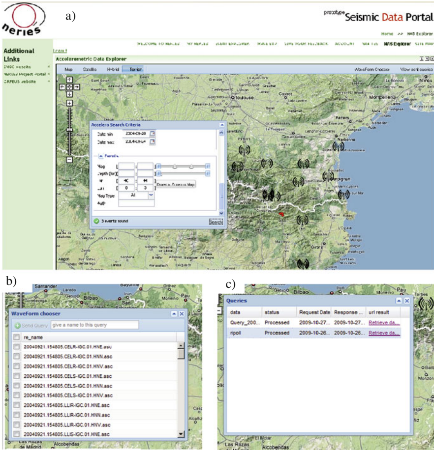
Fig. 9.6 Example of a request to the acceleration data explorer in the seismic data portal with: a the Euro-mediterranean map zoomed in the Pyrenees region, with the epicenters and stations resulting from a query “Accelero Search Criteria”; b the list of records available (“Waveform Chooser”); and c status of the download process (“Queries”)
