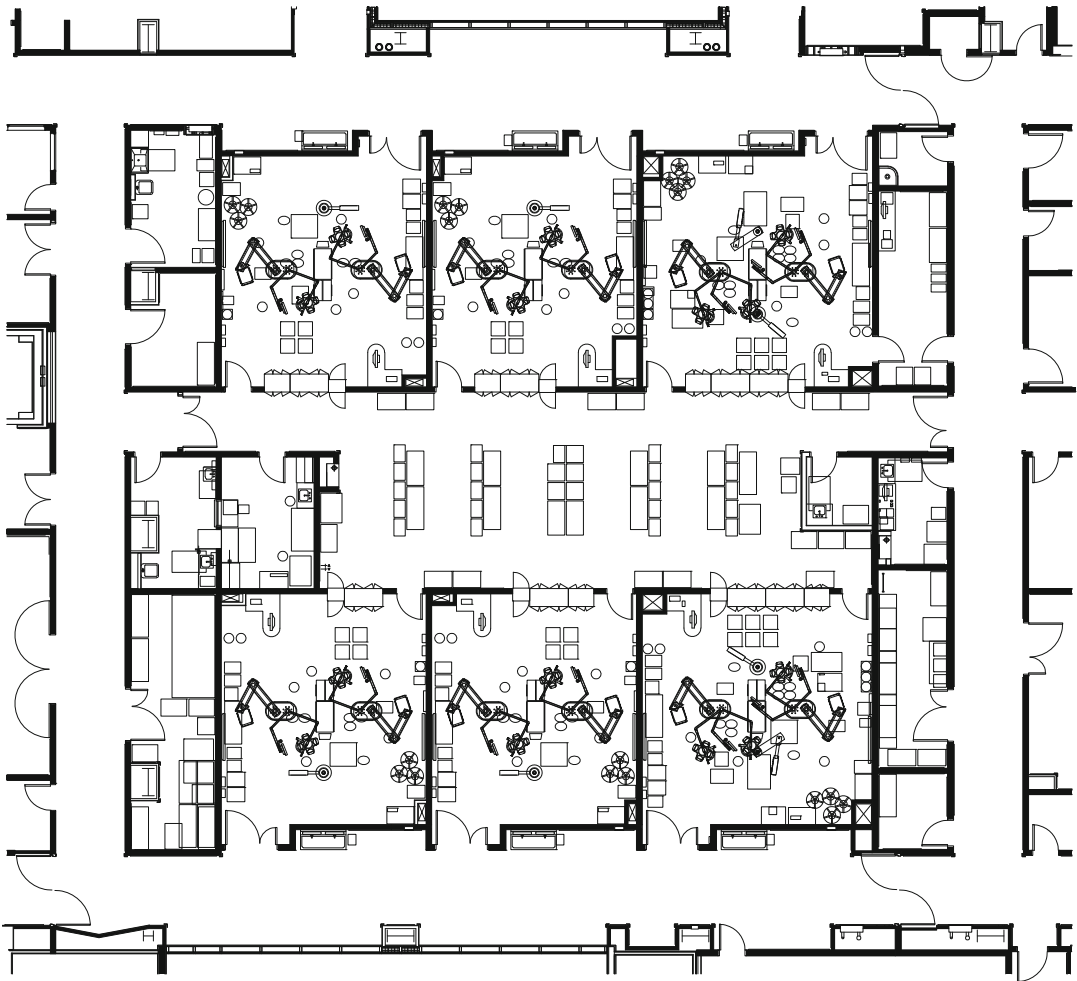
Fig. 34.4 Clean Core Surgical Suite: Six operating rooms organized around a central clean supply core. Architect of Record: Co Architects; Associate Architect: Stantec. (Used with permission from Palomar Pomerado Health. ©2013 PPH)
