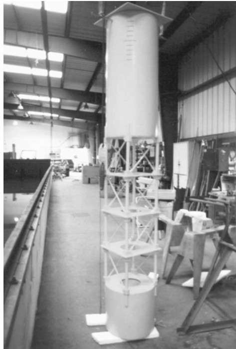
Fig. 1-15. First Truss Spar tested in February 1995 (Courtesy of Technip)
