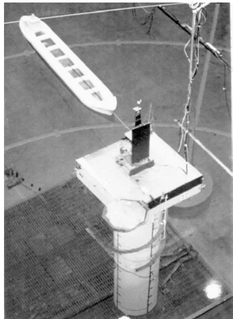
Fig. 1-9. Large-scale model tests conducted in 1993 helped convince Oryx to select the Spar (Courtesy of Technip USA, Inc.)
