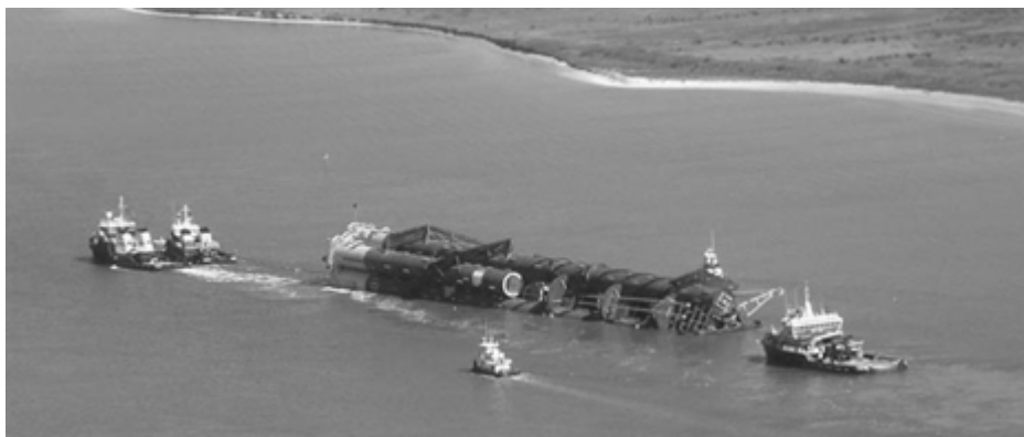
Fig. 1-25. Red Hawk Cell Spar under tow (Courtesy of Technip USA, Inc.)
