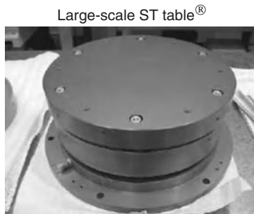
Intended for \phi 8 inch wafer and the A4 size work piece Sphere guide, Air bearing, and Clamping function is provided
