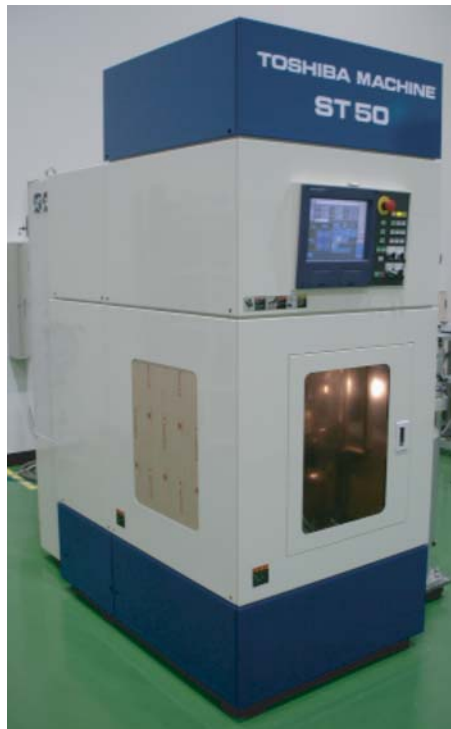
Figure 5.28 Press type of UV nanoimprint tool
