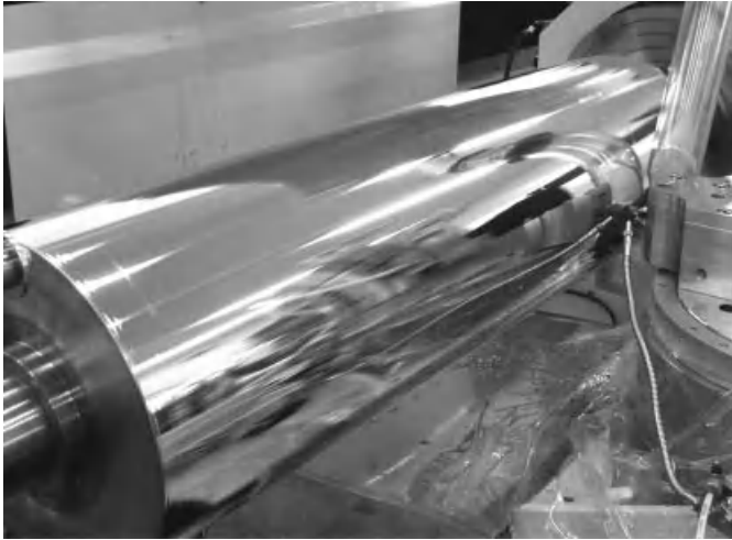
Figure 4.5 V-groove processing of the roll
