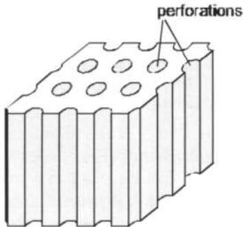
Fig. 21 Schematic diagram of a 2D photonic crystal using anodic porous alumina.
