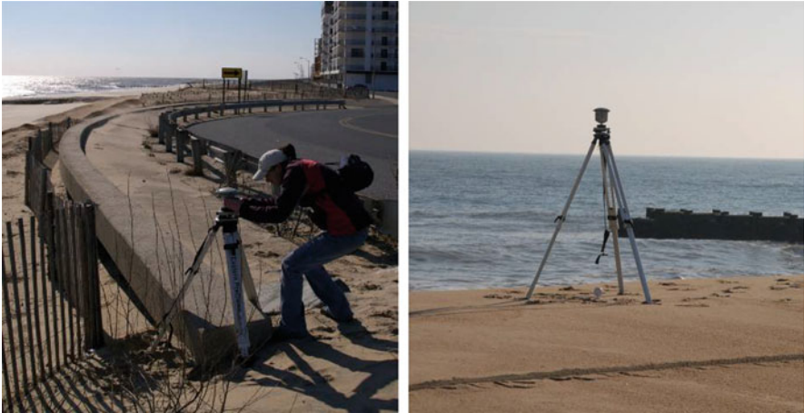
Fig. 3.6 Images depicting GPS surveys of hard structures ( left ) and TLS spherical targets ( right ) used to georeference point cloud collected for these features
