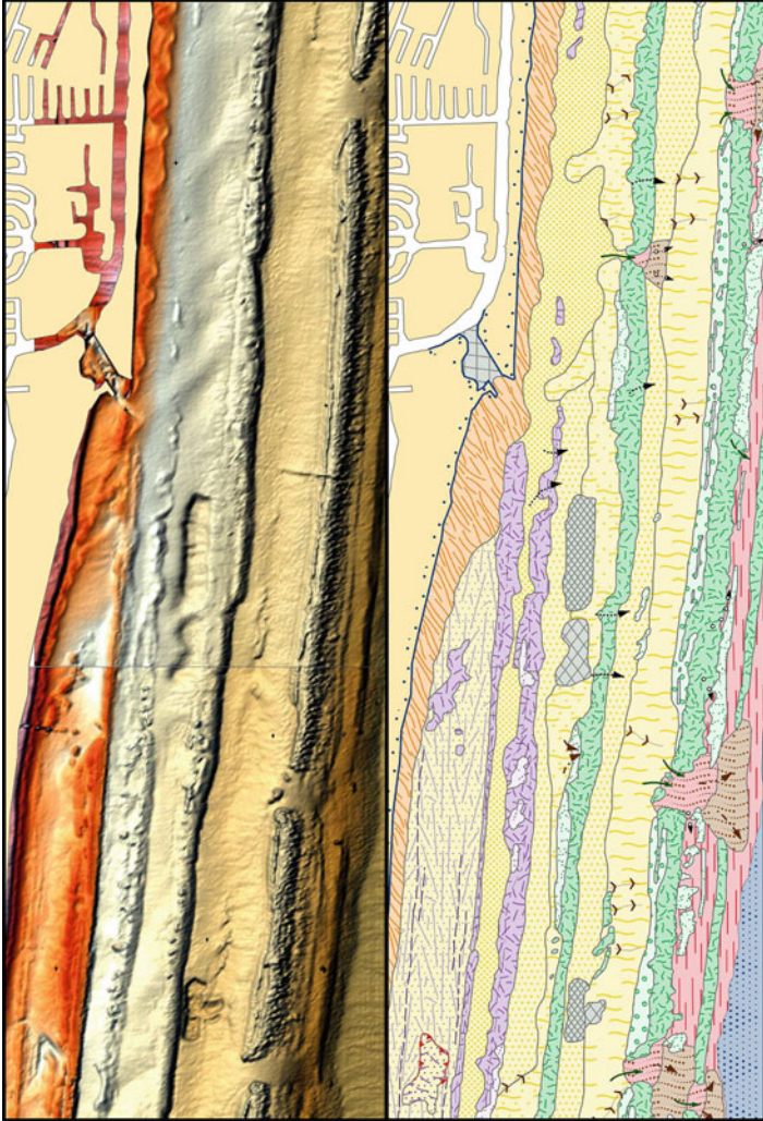
Fig. 2.3 (a) Diptych showing an uninterpreted enhanced LADS image in the left panel and the cognitively interpreted geomorphological units based on bathymetry in the right panel for the southeast Florida continental shelf (see Fig. 2.1 for overall survey location). The raw LADS image was enhanced, vertically exaggerated, and bathymetrically colorized for easier interpretation. Symbols explained in Fig. 2.2 are used to depict the coral reef systems of the Florida Reef Tract and displayed in GIS format using IDRISI. (b) Legend to accompany (a), showing mapping units displayed in the right panel of the diptych in (a). Although this example of mapping units is incomplete as it only refers to the field of view in (a), it demonstrates an ability to interpret LADS bathymetry with symbols specifically developed for depicting submarine topographic units in a GIS format
