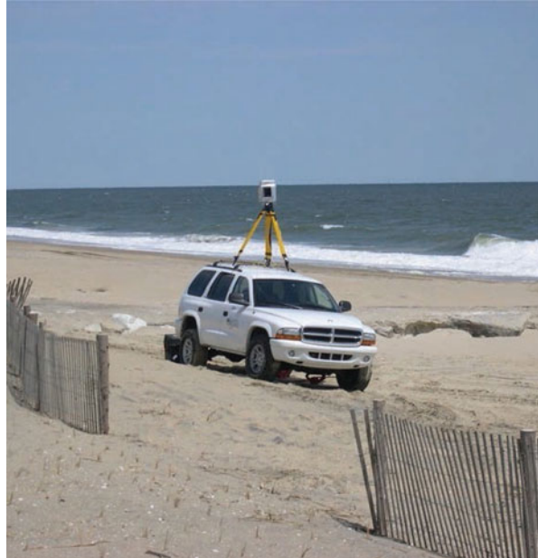
Fig. 3.2 An example of elevating a TLS using a vehicle stabilized with jacks
