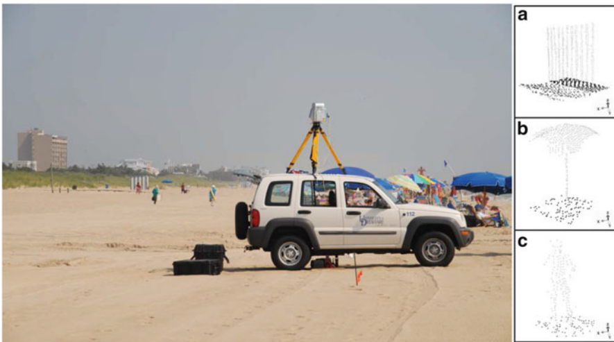
Fig. 3.7 An image depicting many of the non-terrain objects that may be included in TLS surveys in populated regions with point cloud examples of a (a) fence, (b) beach umbrella, and (c) a person
