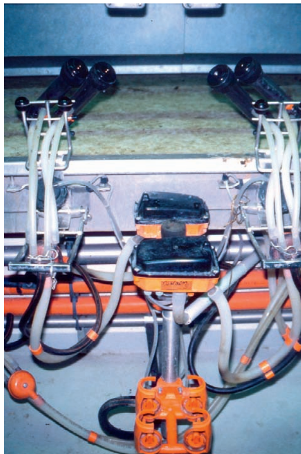
Figure 11 Two units with automatic teat-cup valves and automatic cluster removal (ACR).
