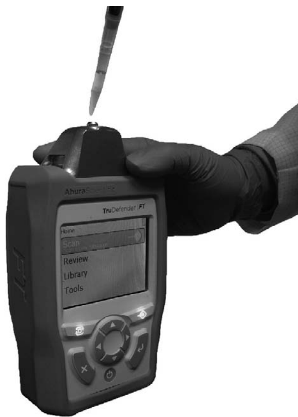
Figure 7 TruDefender™ FT handheld FT-IR (copyright Ahura Scientific, Inc., Wilmington, MA, USA).
