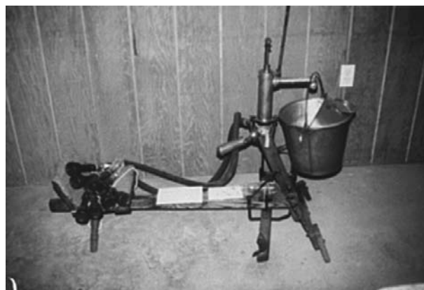
Figure 9 The foot-powered Mehring milker, Maryland (1895).
