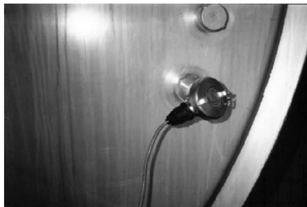
Figure 1 Fiber-optic CoAguLite™ probe inserted through the wall of a commercial cheese vat for the online monitoring of rennet-induced gelation of milk.
