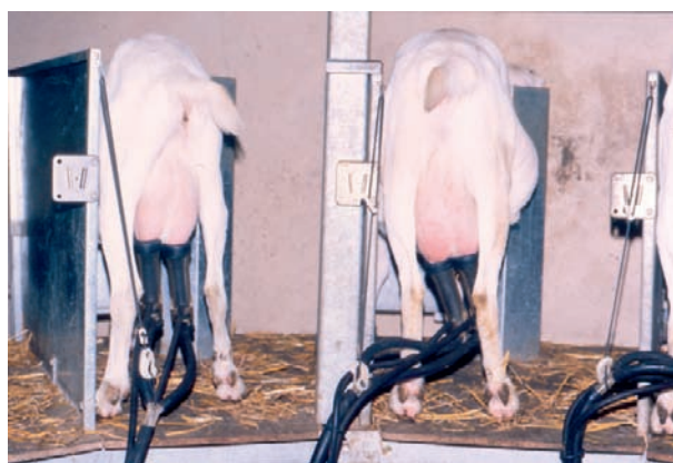
Figure 10 Milking units with automatic teat-cup valves.
