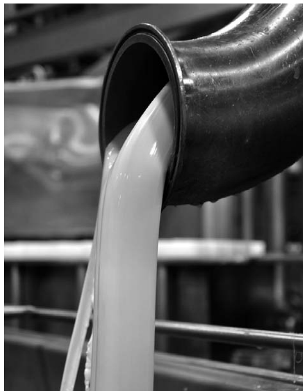
Figure 7 Hot homogeneous mass of cheese as it exits the cooker/stretcher.
