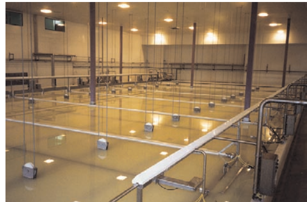
Figure 15 Deep brining system. Courtesy of Fonterra Cooperative Group, New Zealand.
