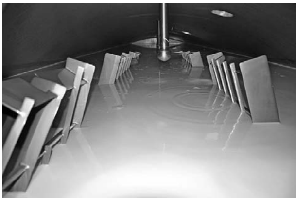
Figure 3 Formation of the initial curd after renneting of milk inside an enclosed cheese vat.
