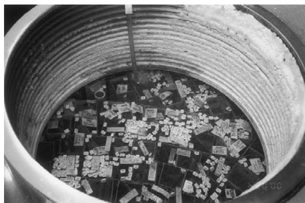
Figure 2 A tank of liquid nitrogen capable of holding 100 000 straws of frozen semen at –196 °C until they are distributed for use worldwide.
