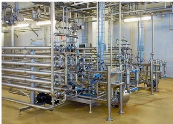
Figure 12 Spiral-tube heat exchanger.
