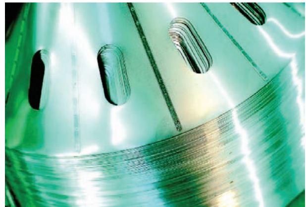
Figure 4 Separator disk stack.
