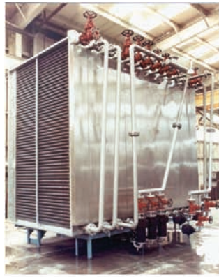
Indirect steam-heated air heater
