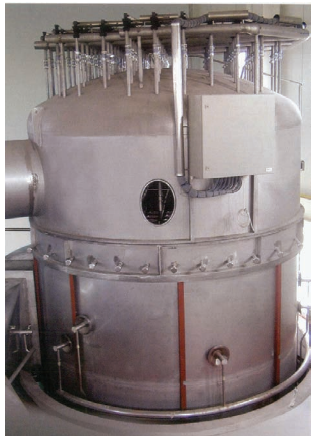
Figure 20 SANICIP™ CIP-able bag filter.
