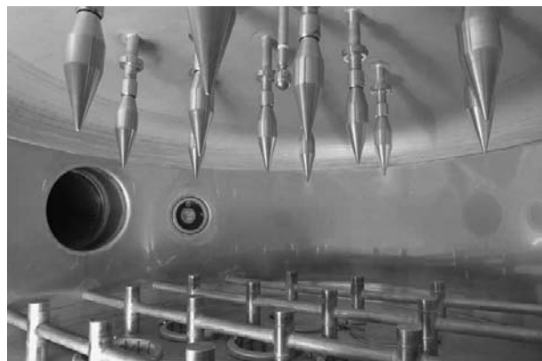
Figure 21 Reverse-jet air nozzle.
