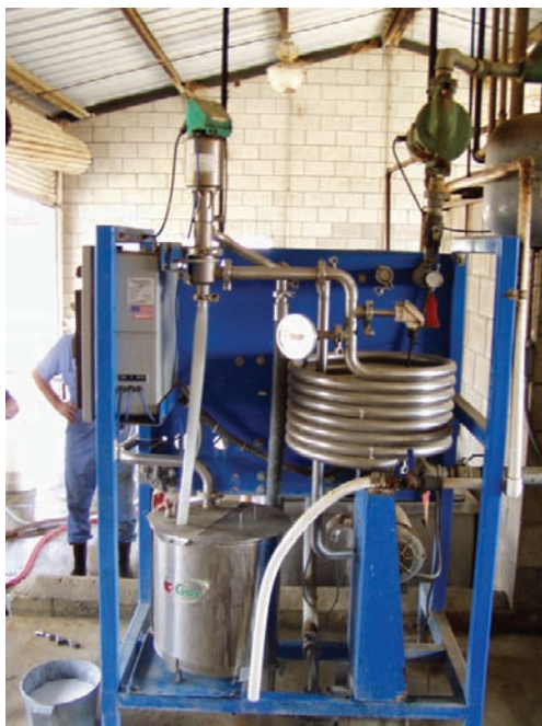
Figure 2 Example of high-temperature short-time pasteurizer (Goodnature, Orchard Park, NY).
