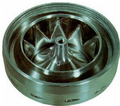
Figure 16 Inside shape of a nozzle bowl.
