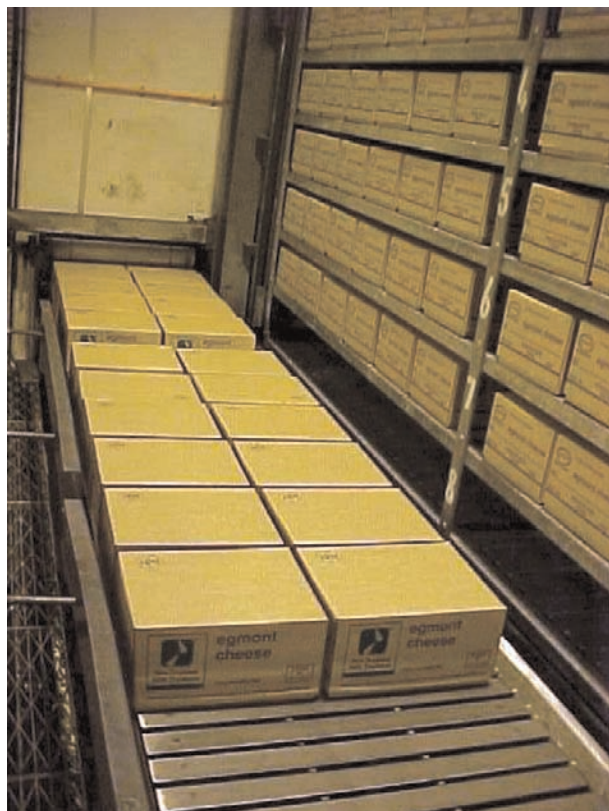
Figure 10 Rapid cooling tunnel. Courtesy of Fonterra Cooperative Group, New Zealand.
