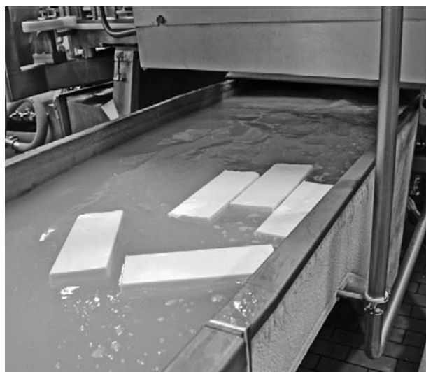
Figure 9 Blocks of LMPS Mozzarella cheese entering the brining system for cooling and salting.
