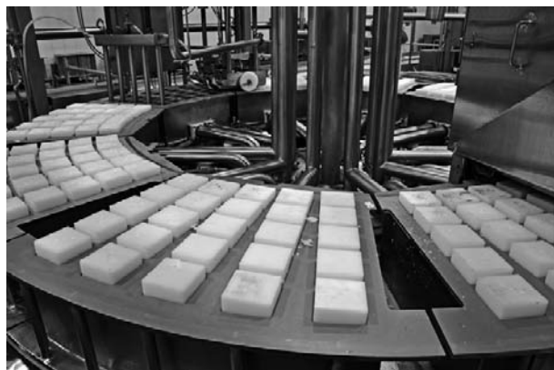
Figure 8 Mechanical molding of hot cheese into rectangular blocks.
