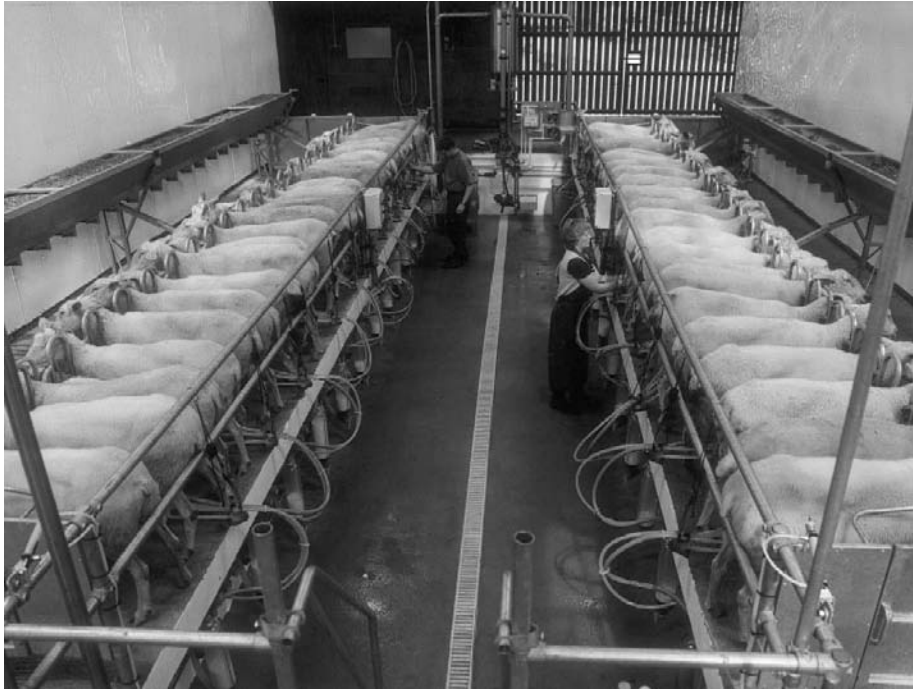
Figure 5 An Alfa Laval double abreast system casse milking parlor, showing automatic feed troughs, individual milk recording jars and low-line milking.
