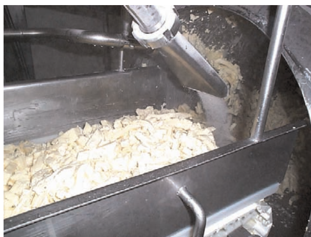
Figure 7 Trommel salting system. Courtesy of Fonterra Cooperative Group, New Zealand.
