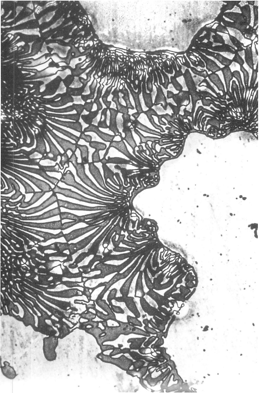
Beryllium-iron alloy draws its strength from the interplay of two contrasting materials.
