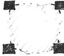
Not helping: when the bay has square columns, the columns eat into the space of the bay; the bay is less coherent.
