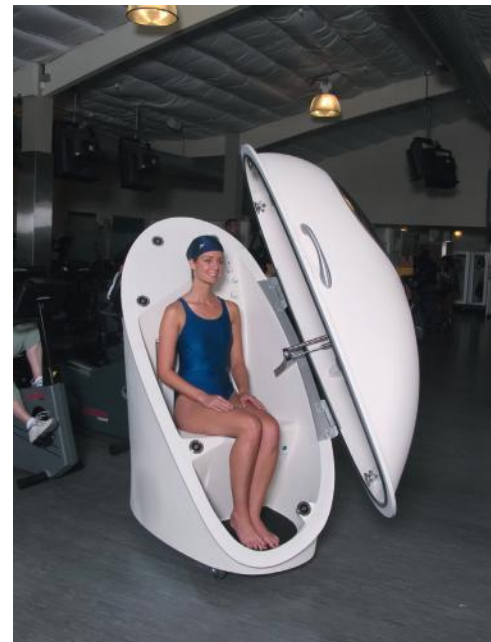
FIGURE 7-6 The BOD-POD measures body fat and fat-free mass. (Courtesy COSMED USA, Inc., Concord, CA.)
