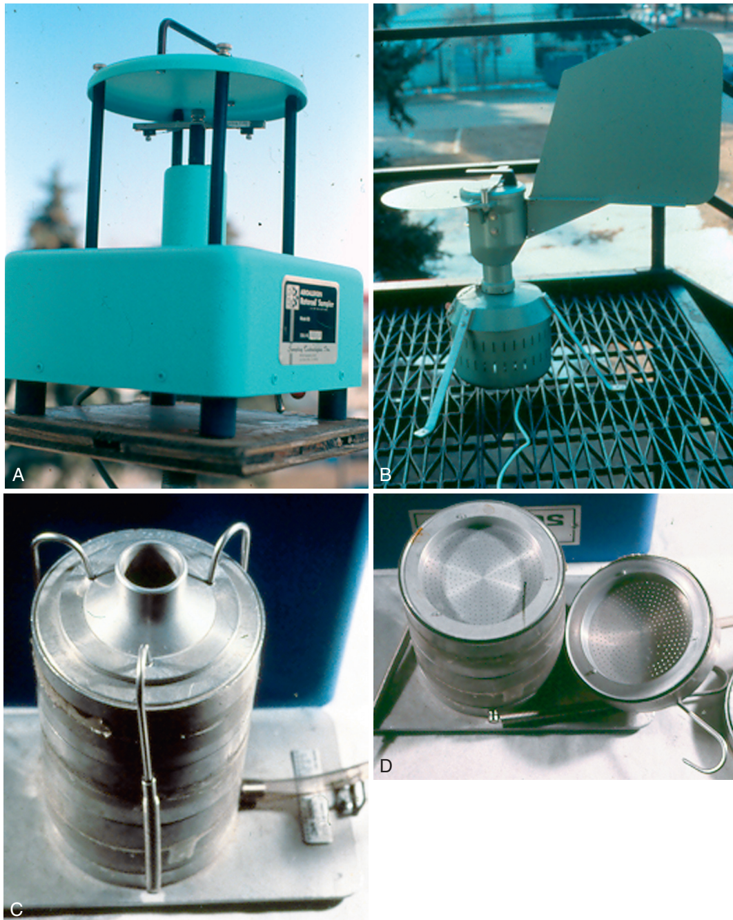
Figure 20-1 Aeroallergen samplers. A – Rotorod; B – Burkard spore trap; C – Andersen cascade impactor; D – Andersen sampler showing inner layers.
