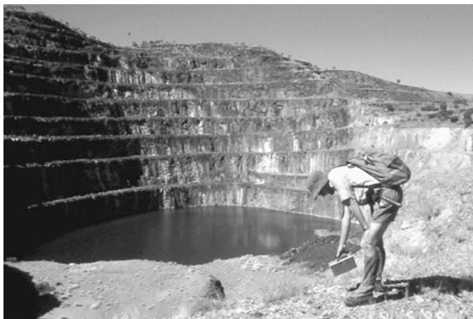
Fig. 6.1 Open pit of the Mary Kathleen uranium mine, Australia. Elevated gamma-ray readings in the open pit correspond to exposed ore lenses, the former haul road, and abandoned ore stockpiles (up to 16 mSv per year). Wallrock oxidation of reactive sulfides produces acidic solutions, yet buffering reactions prevent low pH conditions from developing. The open pit lake contains saline surface waters at a pH of 6.11 (salinity 0.15%; elevated Ca, \text{SO}_4 , Cu, Fe, Mn, Ni, U and Zn values)
