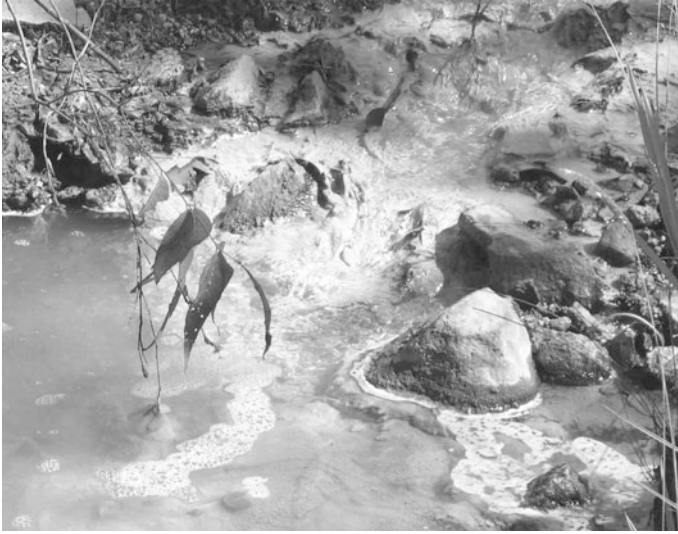
Fig. 3.16 Aluminium hydroxide phases floating as freshly formed white froth on AMD waters (Herberton tin tailings dam, Australia)
