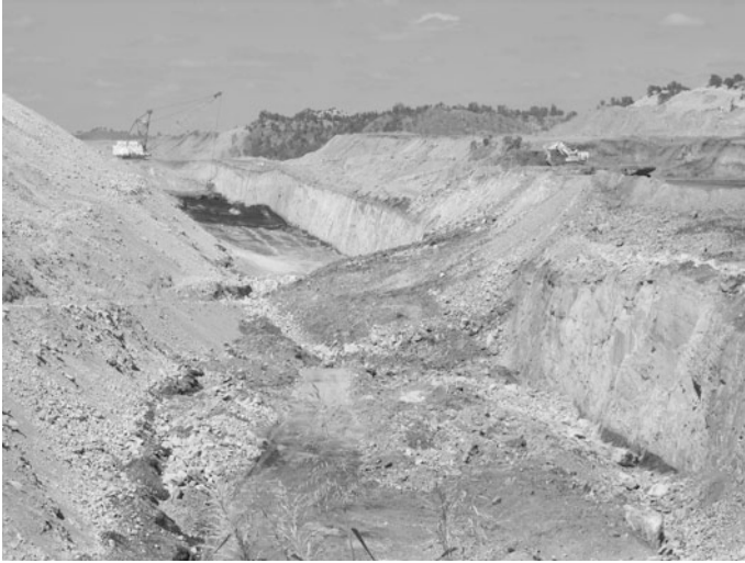
Fig. 2.5 Open cut and spoil heaps of the Moura coal mine, Australia. Spoils of the Moura coal mine are largely non-acid generating due to the lack of pyrite
