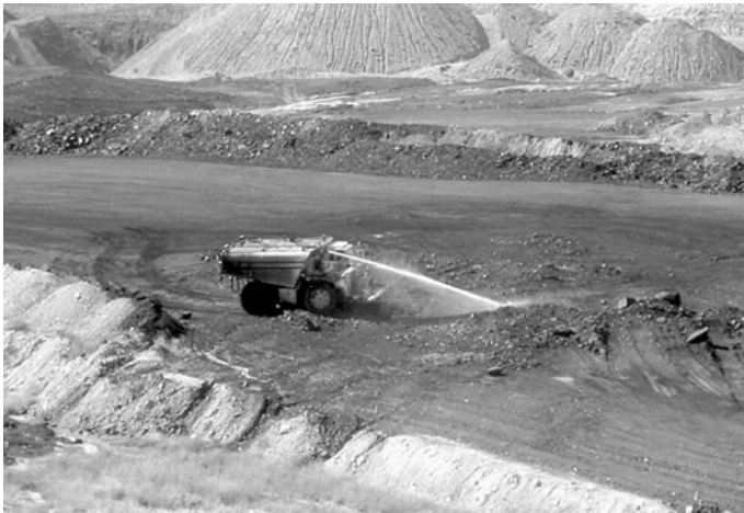
Fig. 2.6 Water spraying of spontaneous combustion at the Blair Attol coal mine, Australia (Photo courtesy of P. Crosdale)
