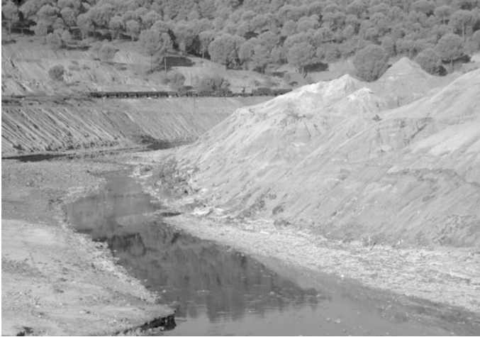
Fig. 2.21 Erodible waste rock dumps at the historic Rio Tinto mines, Spain. Erosion leads to the dispersion of ore and waste particles into the Rio Tinto
