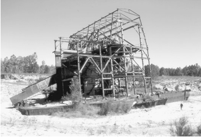
Fig. 1.8 Abandoned tin dredge in the dry stream bed of Nettle Creek, Innot Hot Springs, Australia. The bucket dredge was used in the 20th century to extract alluvial cassiterite. During mining, the dredge caused a massive increase in suspended sediment loads and the deterioration of stream water quality. Consequently, the Mining Act Amendment Act 1948 was introduced which is one of the first pieces of Australian legislation specifically concerned with environmental protection. The act required operators to construct settling ponds for turbid mine waters
