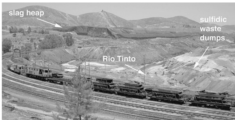
Fig. 3.1 Slag heap, sulfidic waste dumps, and abandoned railway carriages at Rio Tinto, Spain. Mankind has exploited the Rio Tinto ores since the Copper Age 5000 years ago. The mining activities have left uncountable waste rock heaps, ore stockpiles, tailings dumps, slag deposits, and settling ponds, most of which do not support any vegetation. The exploitation of sulfidic ores has created a unique mining landscape and caused massive AMD flowing into the Rio Tinto
