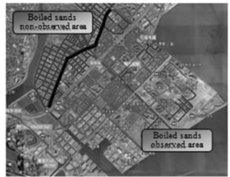
Figure 8. Boiled sands observed/non-observed areas in Urayasu city (Kanto Regional Development Bureau, MLIT, 2011).
