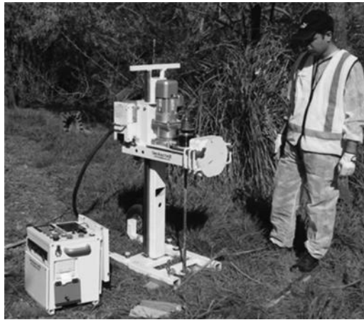
Figure 3. Screw Driving Sounding (SDS) equipment.
