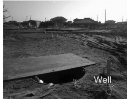
Figure 16. In-situ test to demonstrate the effect of drain pipes in Kamisu City.
