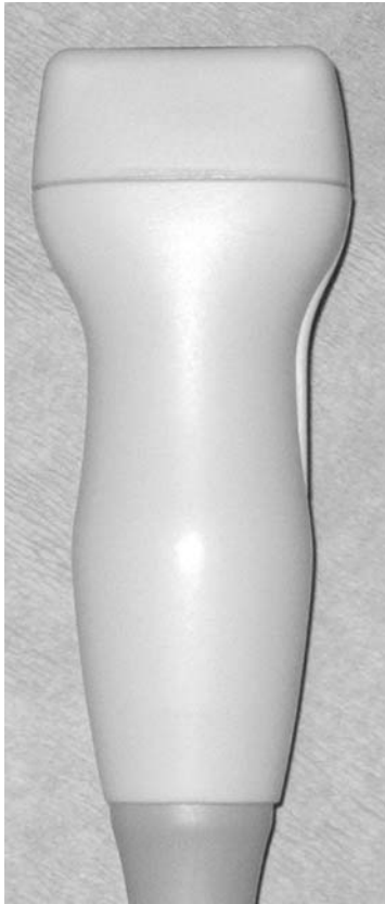
Figure 13.8. Phased array transducer.
