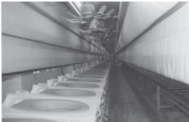
Drying green toilet at Sphinx sanitary (by J.Aarsen).
