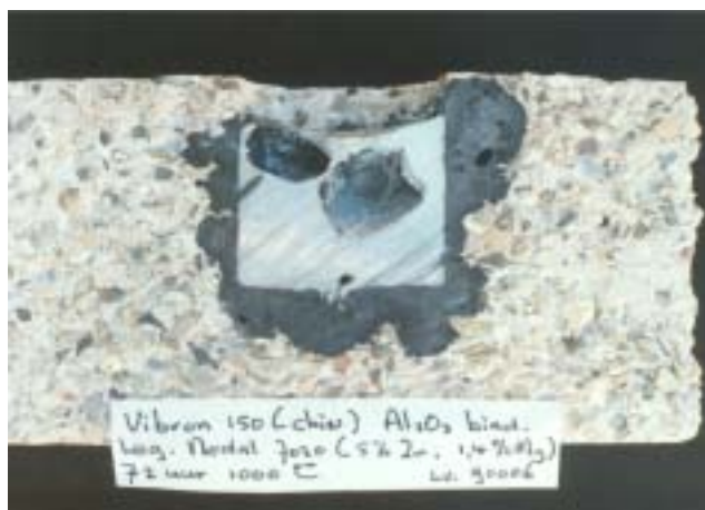
Result of a aluminium cup test (by Gouda Vuurvast, Netherlands).
