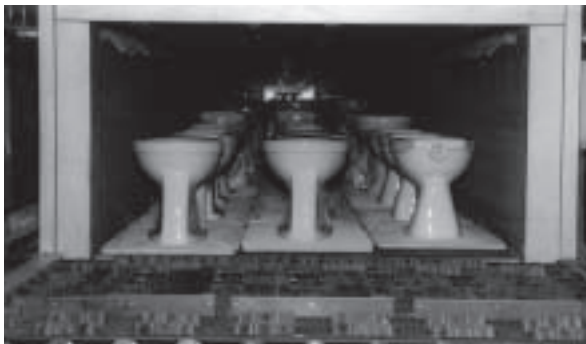
Closets in the oven at Sphinx sanitary (both pictures by J. J.Aarsen).
