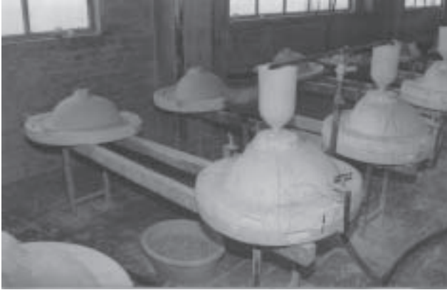
Pouring clay suspension in a mould for producing a wash basin at Sphinx sanitary (by J.Aarsen).
