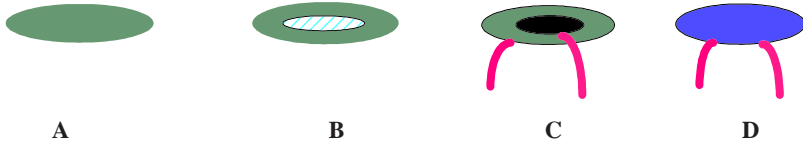
Fig. 11.4.21 The construction of a ceramic capacitor.
