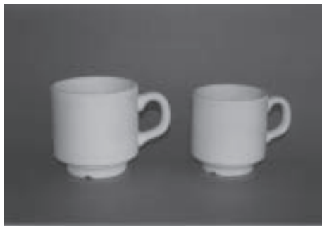
Coffee cup before (left) and after (right) firing (by : E.Bormans)
