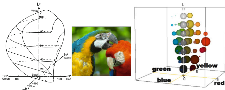
Fig. 1 The CIE L^*a^*b^* color space ( left ) and an example of a color intensity histogram ( right ) of a macaw picture ( middle )
