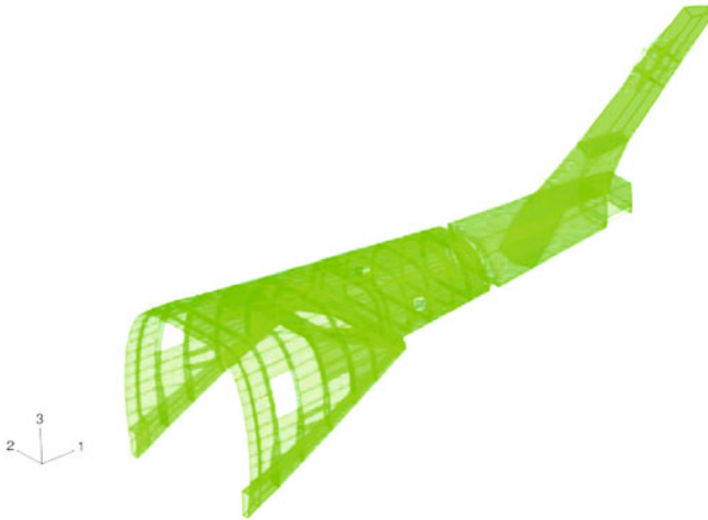
Fig. 1 Translucent view of the finite element model of the rear fuselage. The stringers and ribs are visible
