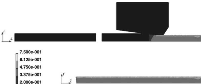
Fig. 3 Finite element simulation of the drawing process: the rod before entry into the die ( top-left ); the rod within the die ( top-right ); the cold drawn rod ( bottom ). Contour bands indicate the levels of the equivalent plastic strain
