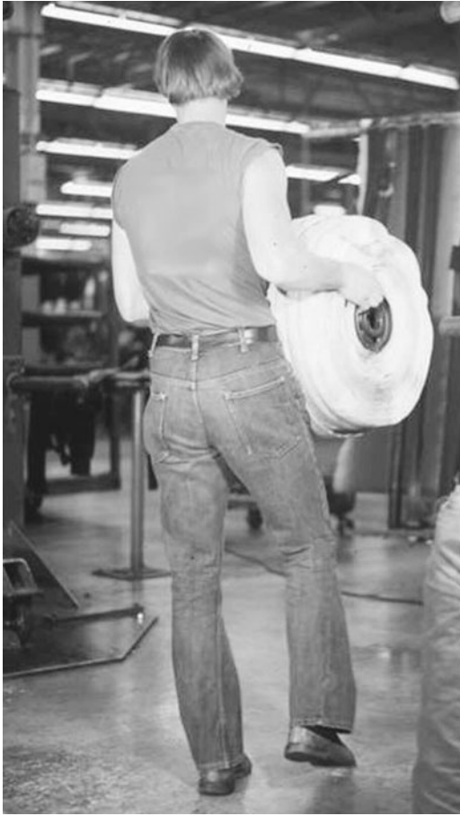
Figure 27-2. The load carried by this worker exceeds 50 kg (110 lb). A mechanical assist device, such as an overhead hoist, would reduce the risk of back injuries on this job. (Photograph by W. Monroe Keyserling.)
