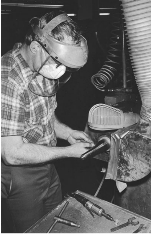
Figure 2-5. Local exhaust ventilation used to protect a worker from asbestos dust generated in working with clutch plates. (Photograph by Earl Dotter.)
