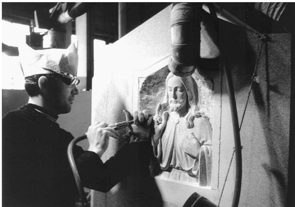
Figure 26-4. Local exhaust ventilation successfully captures dust produced by stone cutting. (Source: W. A. Burgess, Harvard School of Public Health, Boston, Massachusetts.)
