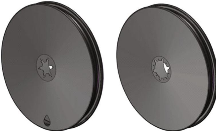
**Fig. 2** *Left and right* side of the IDRA09 wheel rim design
