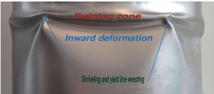
Fig. 8 Buckling mode features
