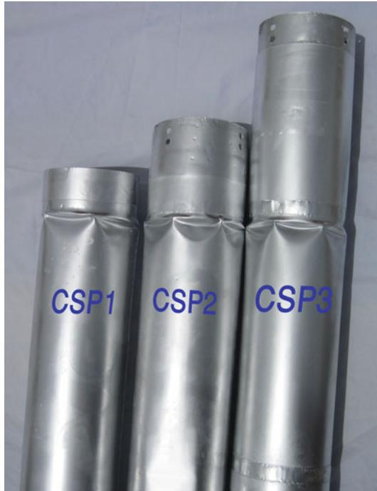
Fig. 7 General buckling mode of the specimens
