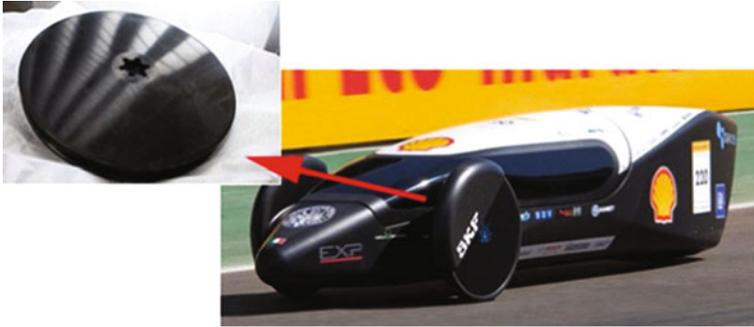
**Fig. 1** Idra09 prototype and its wheel rim
