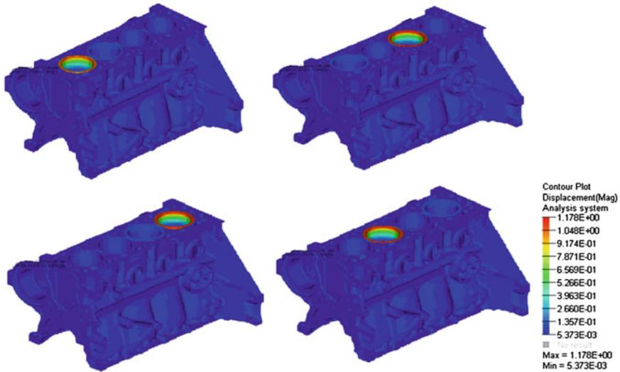
**Fig. 20** Maximum principal tensions—Cylinders 1, 3, 4 and 2 during ignition
