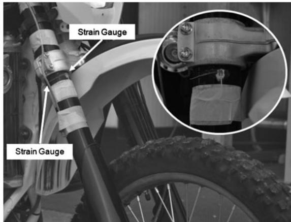
instrumented with four strain gauges placed close to the lower steering plate joint. The strain gauges have been glued to the external surface of the outer tubes, with the main grid axis aligned with the tube axis (Fig. 23).
