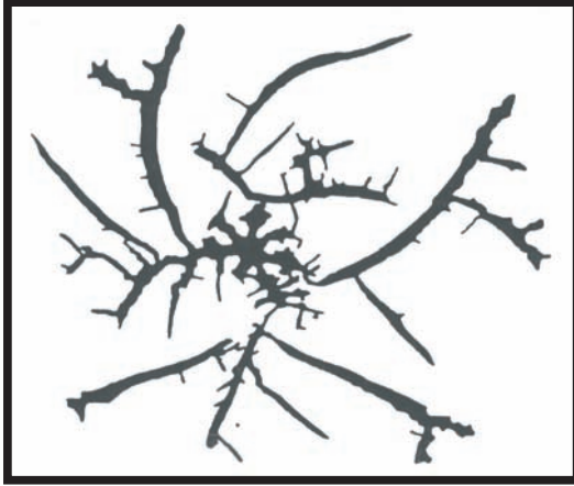
FIGURE 8.29. Fracture pattern in a viscoelastic material (after Van Damme et al. , 1987a).
