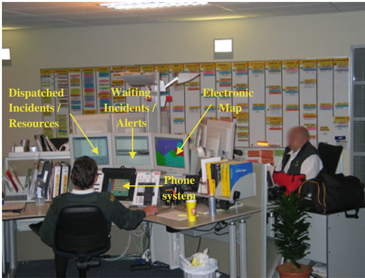
Fig. 3 Cluster of three dispatcher stations at NRCC with whiteboard in background, allowing dispatchers to easily share information when required. Components of dispatcher CAD system are labelled (adapted from Hayes 2006)
