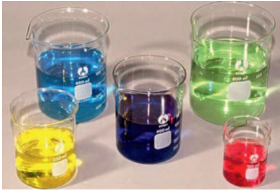
Borosilicate glass (Pyrex) is used for ovenware and chemical equipment.
