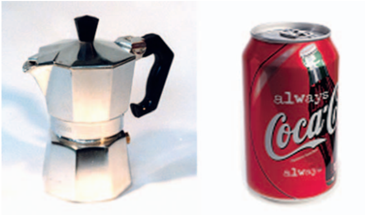
Cast and wrought aluminum alloys, examples of the wide range of properties of this, the most widely used light alloy.
