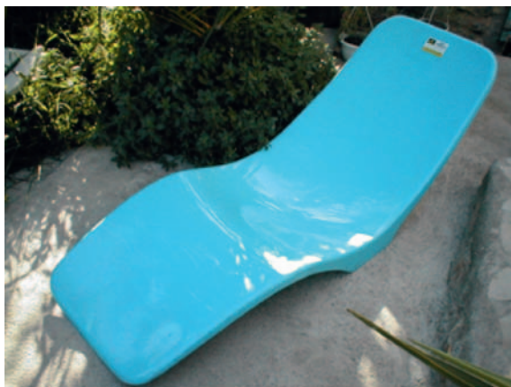
Thermosetting polyester is used as the matrix of this glass-reinforced deck chair.
