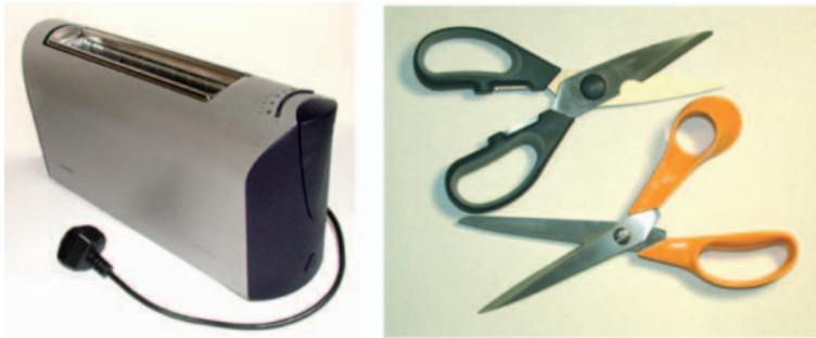
On the left: siemens toaster in brushed austenitic stainless steel (by Porsche Design). On the right, scissors in ferritic stainless steel; it is magnetic, whereas austenitic stainless is not.
