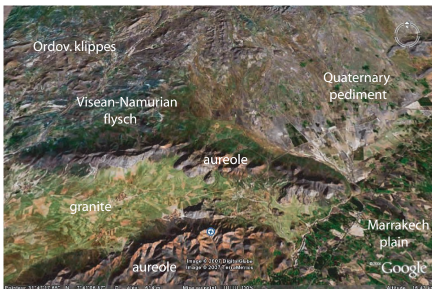
Fig. 3.28 The Ouled Ouaslam laccolith of granite in the eastern Jebilet massif (slightly tilted Google Earth satellite view). The tongue-shaped laccolith grew eastward from a western injection zone located along an early fault (not shown). However, the granite emplacement predates the main, synmetamorphic folding phase (Boummane & Olivier, 2007)
