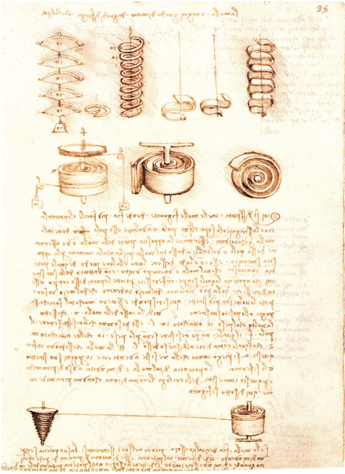
Fig. 2.7. Madrid MS I, f. 85 r. Spring morphologies for use as a power source
