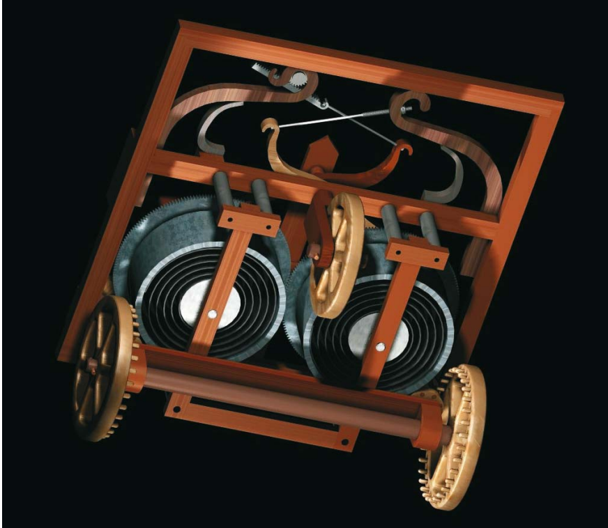
Fig. 2.35. Impetus for the system comes from the springs housed within their barrels
