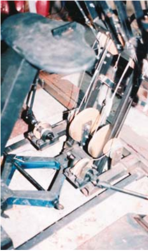
Fig. 3.45. Robot Knight reconstruction for BBC. Leg detail
