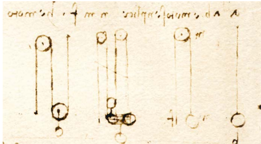
▶ Fig. 3.49. ▶ Codex Arundel 263, f. 42 r. Detail of pulley system
