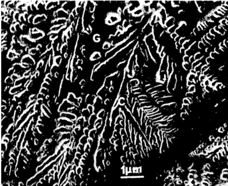
Fig. 3.4 SEM image of a polished section of slag. Crystals C of merwinite and glass G in dendritic form [6]
