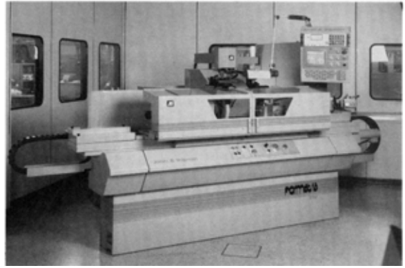
Figure 14.44 A CNC cylindrical grinding machine. (Courtesy of Jones and Shipman Ltd)
