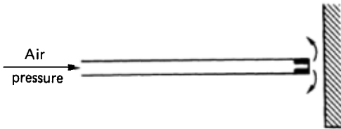
Figure 17.59 The principle of air gauges
