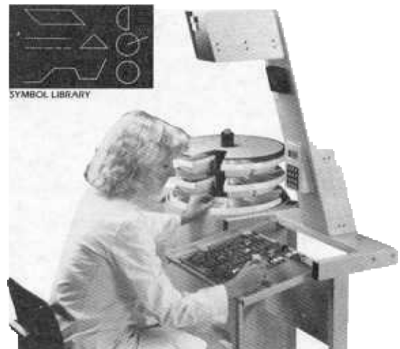
Figure 7.2 Assembly of components using an assembly director
