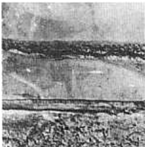
Figure 1.37 Example of 'knife-line' attack on stainless steel welds. (Courtesy of ICI)
