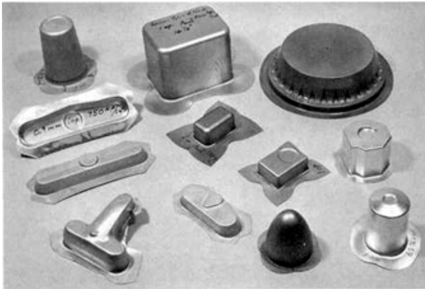
Figure 4.140 (a) Pure hydroforming operation: 1, hydraulic cushion; 2, pressure regulator; 3, cup diaphragm; 4, blank material; 5, pressure pad; 6, punch. (b, c) A range of jet engine and aircraft components. (d) Side panel of a car body. (e) Car parts. (Parts (b) to (e) courtesy of Saab-Scania AB Car Division, Sweden)
