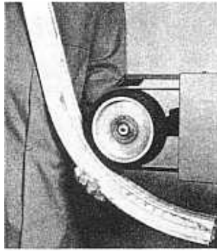
Removal of lines caused by bending of aluminium extrusion
