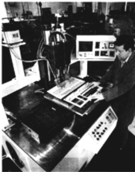
Figure 9.1 PSM Automated Systems new CNC Heatsrter can install up to 45 fasteners per minute and can be preprogrammed in three axes ( x , y and z )
