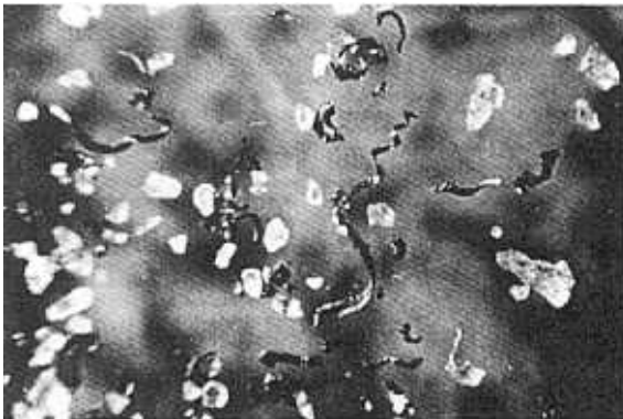
Figure 8.9 Grinding debris showing chips, metal globules and abrasive particles
