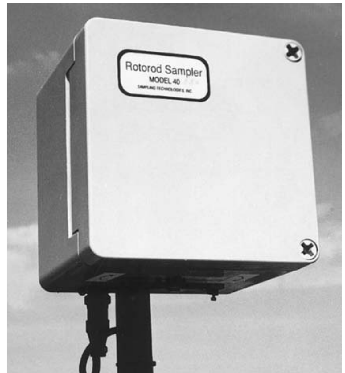
FIGURE 6.1 Rotating impaction sampler: Rotorod sampler model 40 (Sampling Technologies, Minnetonka, MN). (Courtesy of Medical Media Service, Wm. Middleton Memorial Veteran's Hospital, Madison, WI.)
