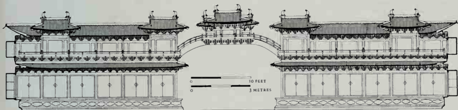
310. Ta-t'ung-fu, Shansi, library of Lower Hua-yen-ssu, sūtra cupboards, façade
