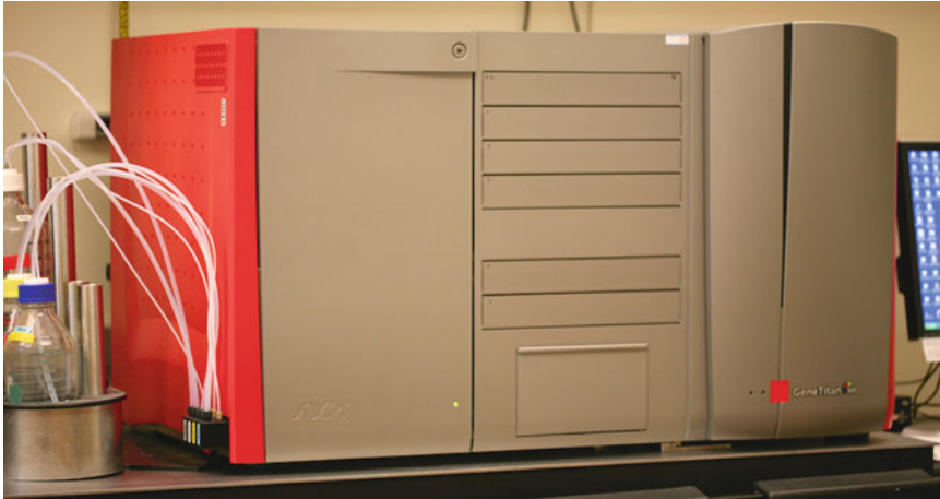
Fig. 3 The GeneTitan system (Affymetrix) used to hybridize, wash, stain and scan labeled samples to Affymetrix 1.1 ST array plates in 16, 24, and 96 Peg array formats
