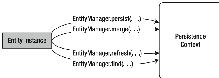
Figure 10-7. A graphical representation of how an entity can be attached to the EntityManager persistence context
