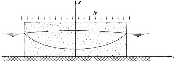
Figure 7.10 *Generation of fresh water reservoir*
