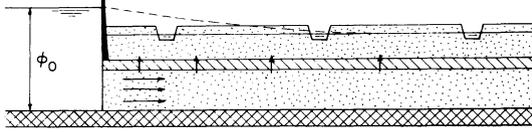
Figure 3.5 One-dimensional flow in semi-confined aquifer
