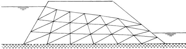
Figure 8.4 Flow through a dam
