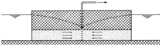
Figure 3.3 Radial flow in confined aquifer
