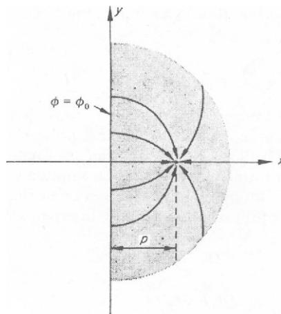
Figure 4.4 *Well near straight impermeable boundary*
