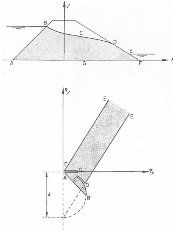
Figure 5.12 *Hodograph for flow through a dam*
