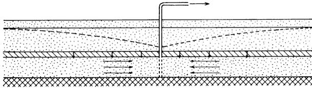
Figure 3.6 Radial flow in semi-confined aquifer
