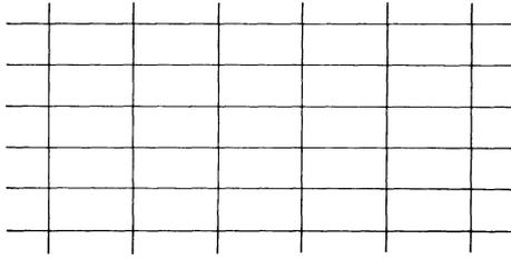
Figure 6.3 *Mesh for finite differences*
