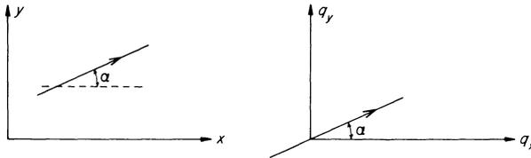
Figure 5.8 *Straight stream line in hodograph*
