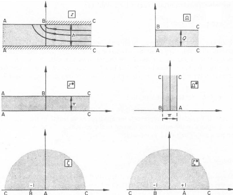
Figure 5.2 Flow in an infinite layer
