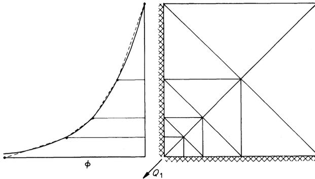
Figure 8.3 Mesh for radial flow
