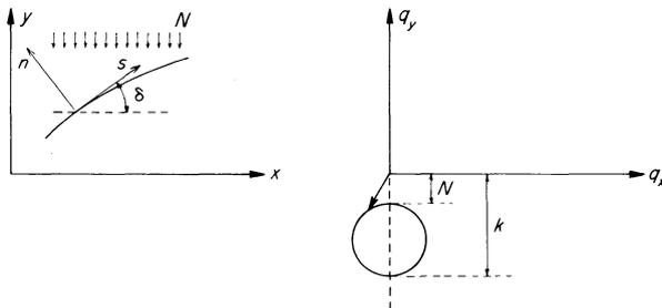
Figure 5.11 Free surface with infiltration in hodograph
