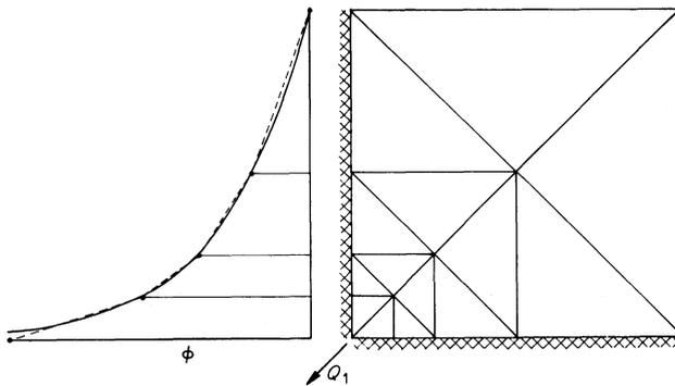
Figure 8.3 Mesh for radial flow
