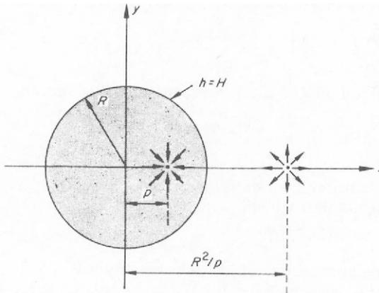
Figure 4.6 Eccentric well in circular aquifer
