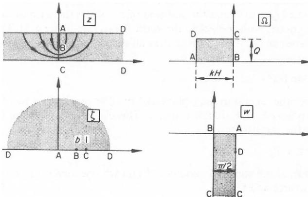
Figure 5.3 Flow under a screen
