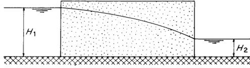
Figure 3.9 One-dimensional flow in unconfined aquifer
