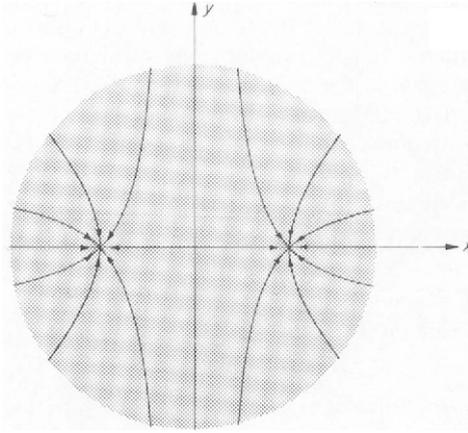
Figure 4.2 Two sinks in confined flow
