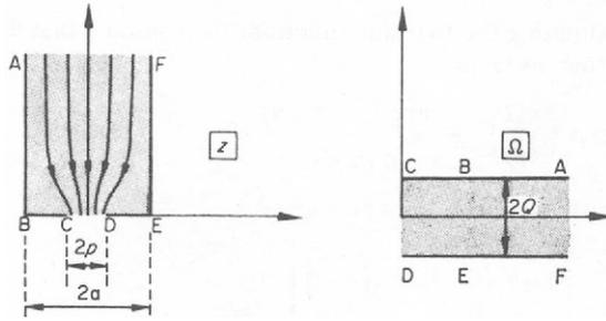
Figure 5.4 Flow through a slit
