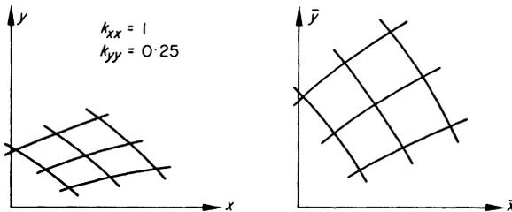
Figure 4.9 *Potential lines and stream lines in anisotropic porous medium*
