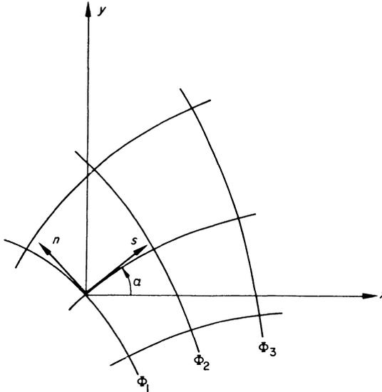
Figure 4.7 *Potential lines and stream lines*
