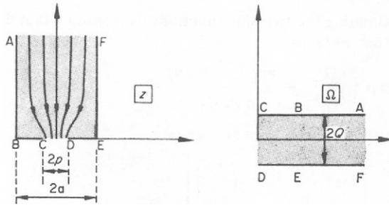
Figure 5.4 Flow through a slit
