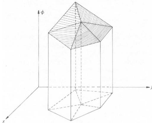
Figure 8.1 *Linear interpolation*
