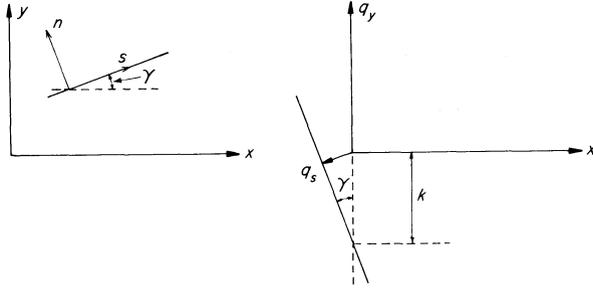
Figure 5.9 *Seepage surface in hodograph*
