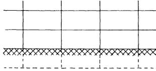
Figure 6.4 *Impermeable boundary*
