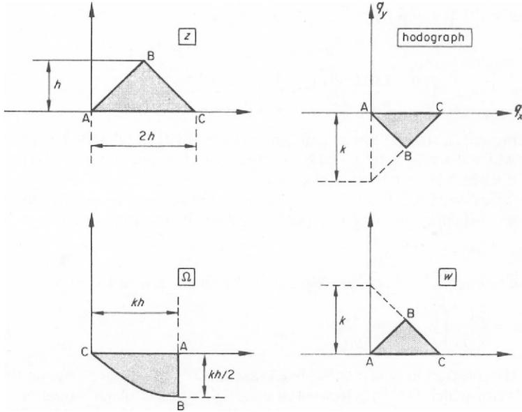
Figure 5.14 Flow in a triangular dam
