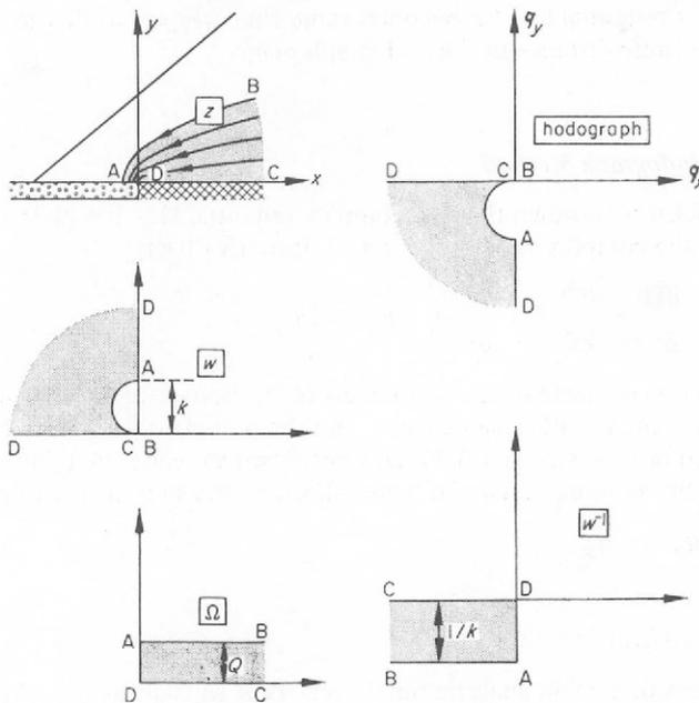
Figure 5.13 Flow in a drained dam
