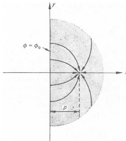
Figure 4.3 *Well near straight canal*
