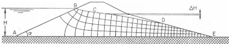
Figure 6.2 Flow net with a free surface
