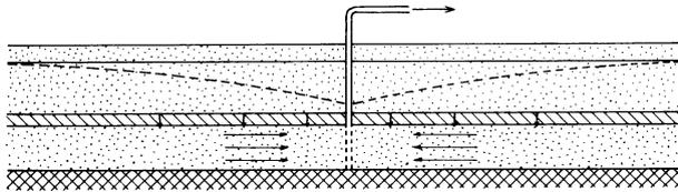
Figure 3.6 Radial flow in semi-confined aquifer
