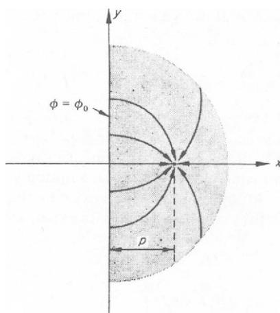
Figure 4.4 *Well near straight impermeable boundary*
