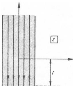
Figure 5.5 Equivalent length of contraction
