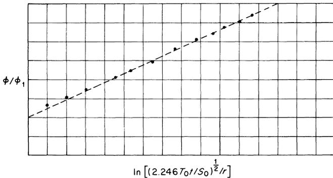
Figure 7.3 *Determination of transmissivity and storativity from pumping test*
