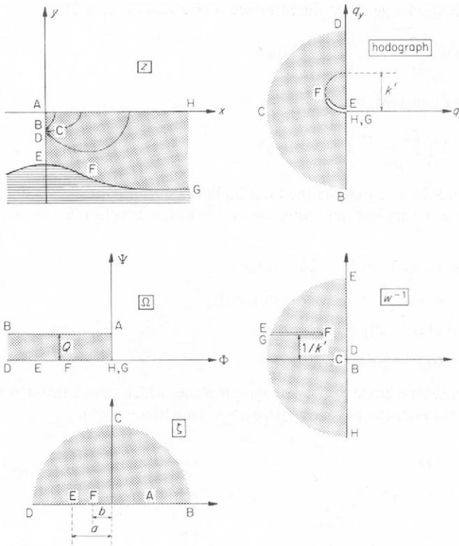
Figure 5.17 Flow towards a drain above an interface
