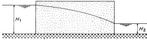
Figure 3.9 One-dimensional flow in unconfined aquifer
