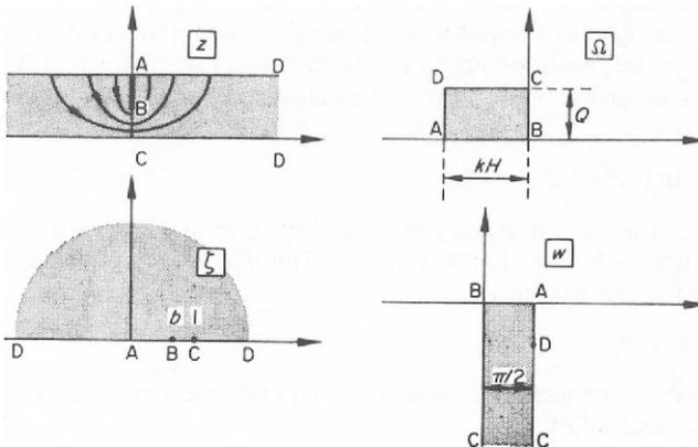
Figure 5.3 Flow under a screen
