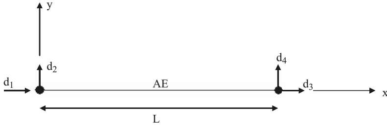
Fig. 6.7. Pinned end of a member
