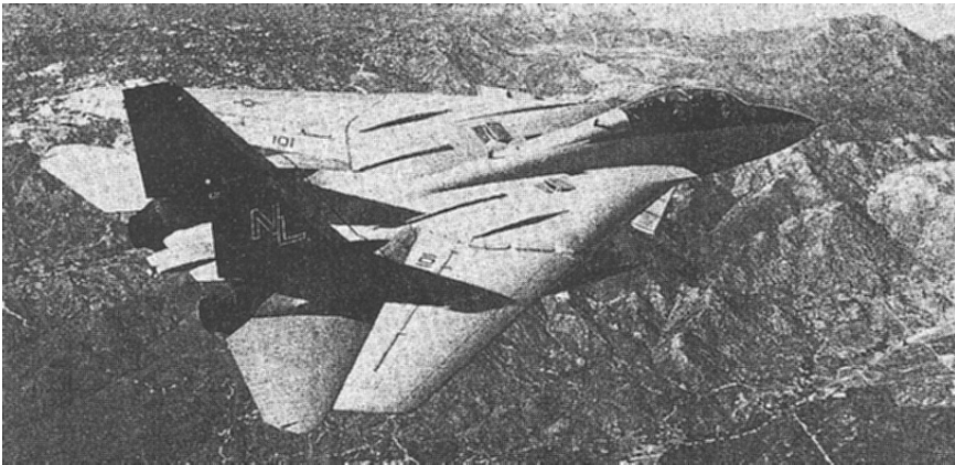
Fig. 2.53. The F-14 with wing and glove movement (courtesy of Grumman Corporation, USA)
