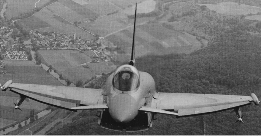
Eurofighter demonstrates the unstable, canard configuration, 'fly-by-wire' FCS and advanced cockpit exhibited by the latest generation of fighters.
