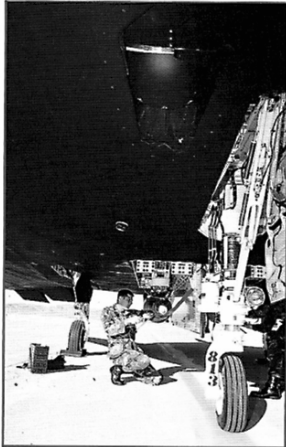
Above: The nose-mounted FLIR sensor is used to search for and acquire the target. The turret cover has serrated edges to reduce radar cross-section and is covered in a fine mesh which acts like a flat surface when illuminated by radar. As a back-up the upper nose turret also has a boresighted laser designator. Both FLIR and DLIR turrets are interchangeable.
