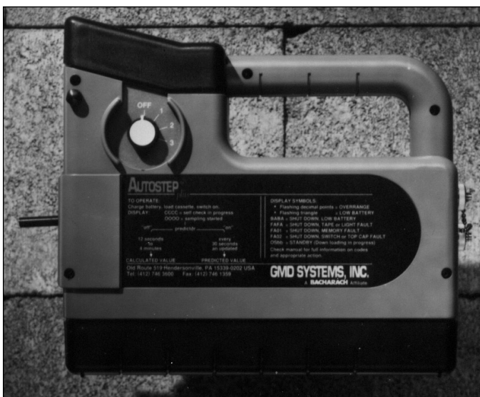
Figure 17-17. A direct-reading, hand-held paper tape instrument for monitoring certain isocyanates. (Courtesy GMD Systems, Inc.)
