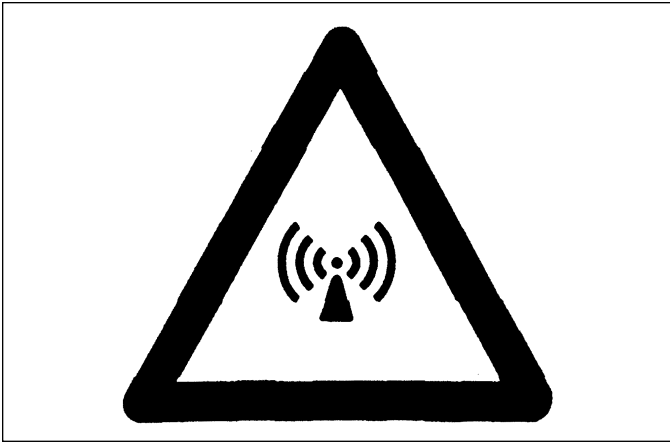
Figure 11-15. The internationally recognized radiofrequency hazard icon, “the radiator.” OSHA has not updated its published radiofrequency standard, but has informed IEEE that it will not cite an organization using this symbol instead of the obsolete symbol found in the OSHA regulations.
