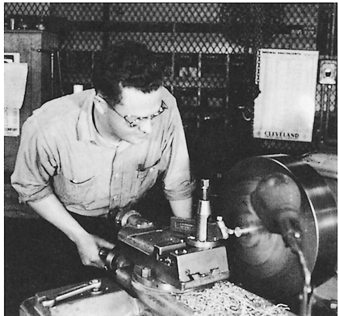
Figure 5-7. Full-cup sideshields are designed to restrict the entry of flying objects from the side of the wearer.
