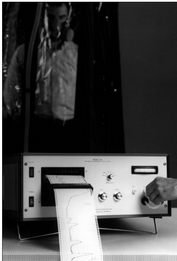
Figure 22-37. A portable corn oil quantitative fit-test system utilizes a test enclosure. (Courtesy Air Techniques Inc.)
