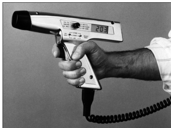
Figure 17-20. A portable hydrocarbon analyzer that uses a photoionization detector. (Courtesy Sentex Systems, Inc.)
