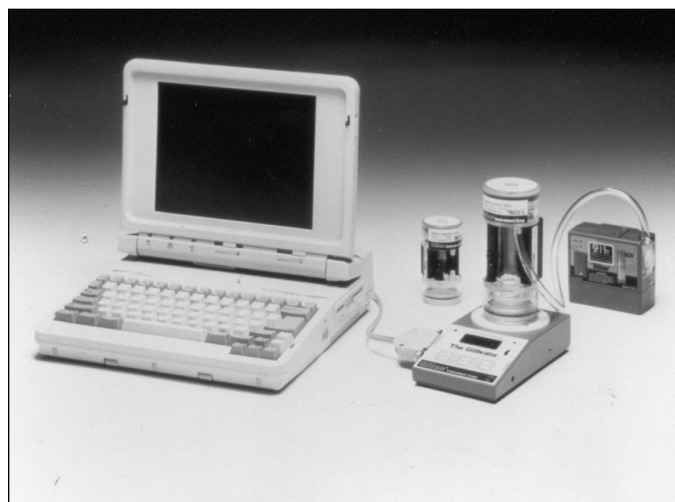
Figure 16-17. Electronic soap-bubble meter provides calibration results quickly and accurately. Calibration information can be stored on a computer database. (Courtesy Gillian Instrument Corp.)
