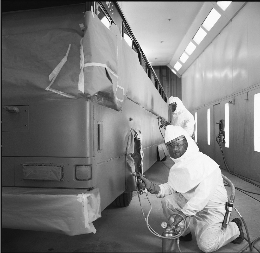
Figure 22–19. Continuous flow air-line respirators are used in conjunction with a compressor system. The manifold for connecting to the air source can be seen in the background. (Courtesy 3M.)
