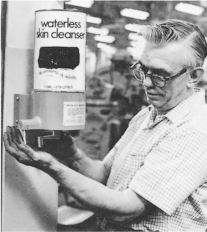
Figure 18–12. Industrial hand cleansers are available as plain soap powders, abrasive soap cakes, liquids, cream soaps, and waterless hand cleaners.
