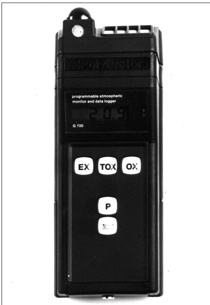
Figure 17-4. A multigas detector that can use a thermal conductivity probe for high concentrations of combustible gases (0-99.9 percent by volume). (Courtesy GfG Gas Electronics, Inc., 200 S. Hanley, St. Louis, MO 63105.)
