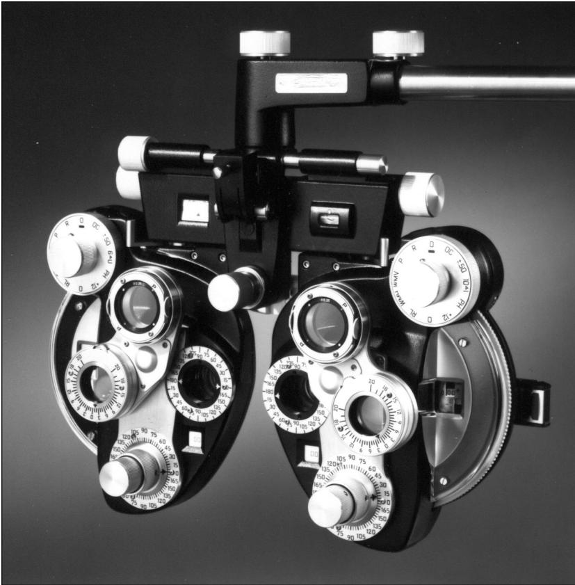
Figure 5-3. A phoropter is used with a set of test lenses to find which ones aid vision. (Photograph reprinted with permission of Reichert Ophthalmic Instruments.)
