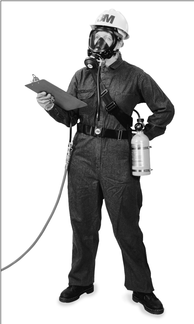
Figure 22–27. Combination self-contained breathing apparatus and air-line respirators can be connected to an external air supply for working in a hazardous atmosphere and still allowing for escape without removing the respirator. (Courtesy 3M.)
