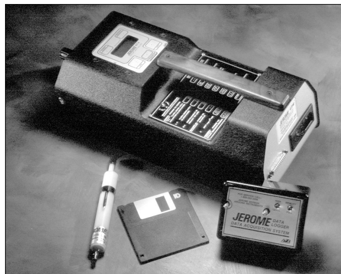
Figure 17–13. An instrument for monitoring mercury vapor based on the conductivity of a gold foil. (Courtesy Arizona Instrument Corporation.)
