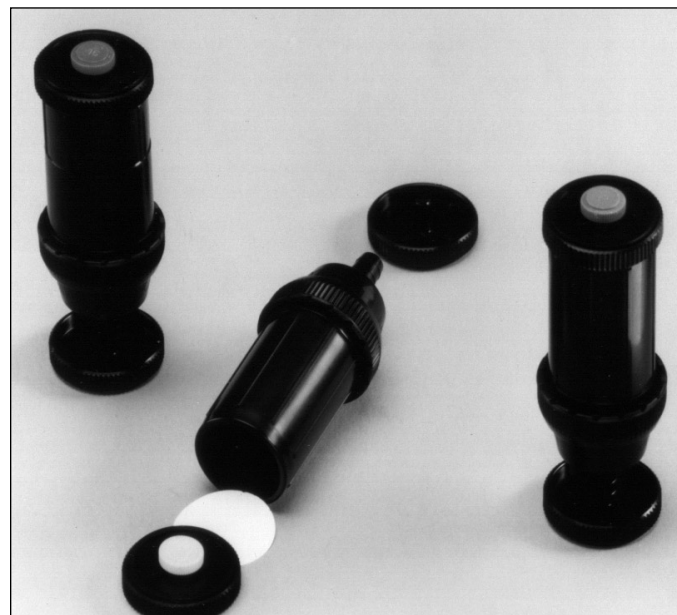
Figure 16–10. Air sampling for asbestos is conducted using a three-piece cassette, a 50-mm black conductive cowl, and a 25-mm filter. (Courtesy MSA.)
