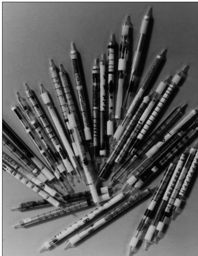
Figure 17–14. Length-of-stain tubes intended for short sampling periods. (Courtesy Draeger Safety, Inc.)
