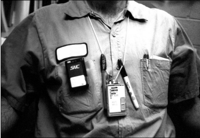
Figure 10–8. A health physics technician wearing a thermoluminescence detector attached to a neck strap and an electronic alarming dosimeter on his right shirt pocket.
