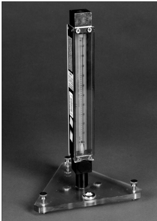
Figure 16-20. A single-column precision rotameter can be used as a secondary calibration device. (Courtesy Fermilab Visual Media Services Dept.)
