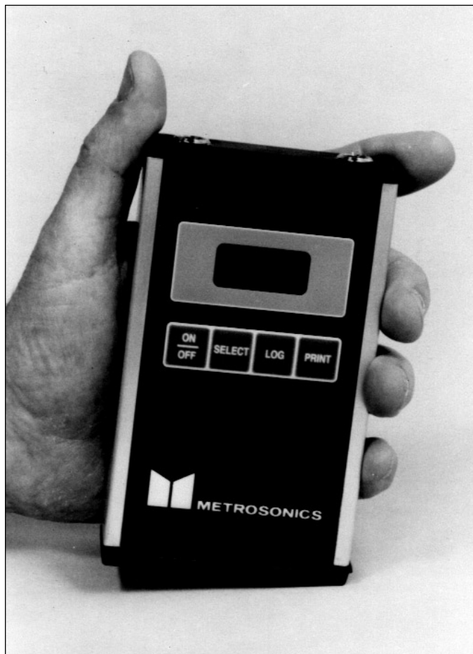
Figure 12–10. Photographs of two commercially available personal monitors developed for heat-stress exposures. (Courtesy of Metrosonics, Inc, and Quest Technologies.)
