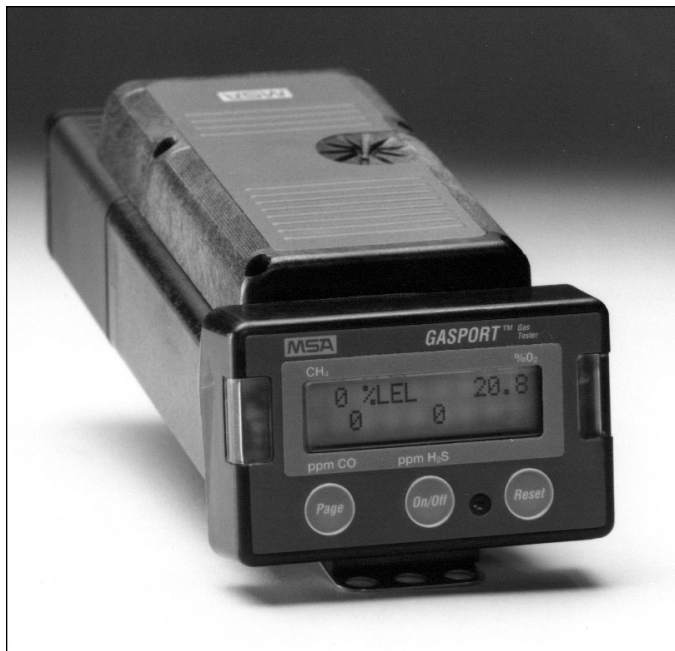
Figure 17-5a. A Gasport® combustable gas monitor. (Courtesy MSA.)
