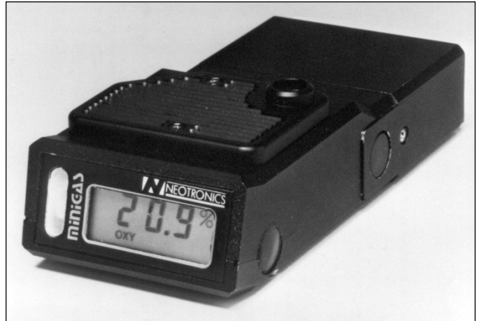
Figure 17-2. A multigas monitor that uses catalytic decomposition to measure combustible gases. (Courtesy Neotronics of North America, Inc.)
