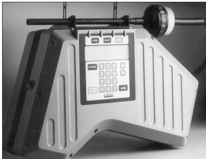
Figure 17–21. A portable, direct-reading instrument with an infrared spectrophotometer. (Courtesy The Foxboro Company.)
