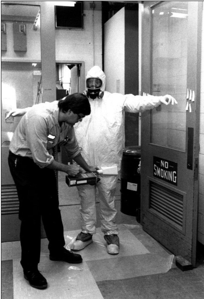
Figure 10–13. Health physics technician monitoring protective clothing after removal of outer protective suit. Survey meter has a dual plastic scintillator to detect alpha-, beta-, and gamma-radioactivity.
