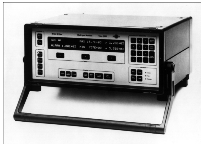
Figure 17-23. A transportable, direct-reading photoacoustic spectrometer using 115 V AC power. (Courtesy California Analytical Instruments, Inc.)
