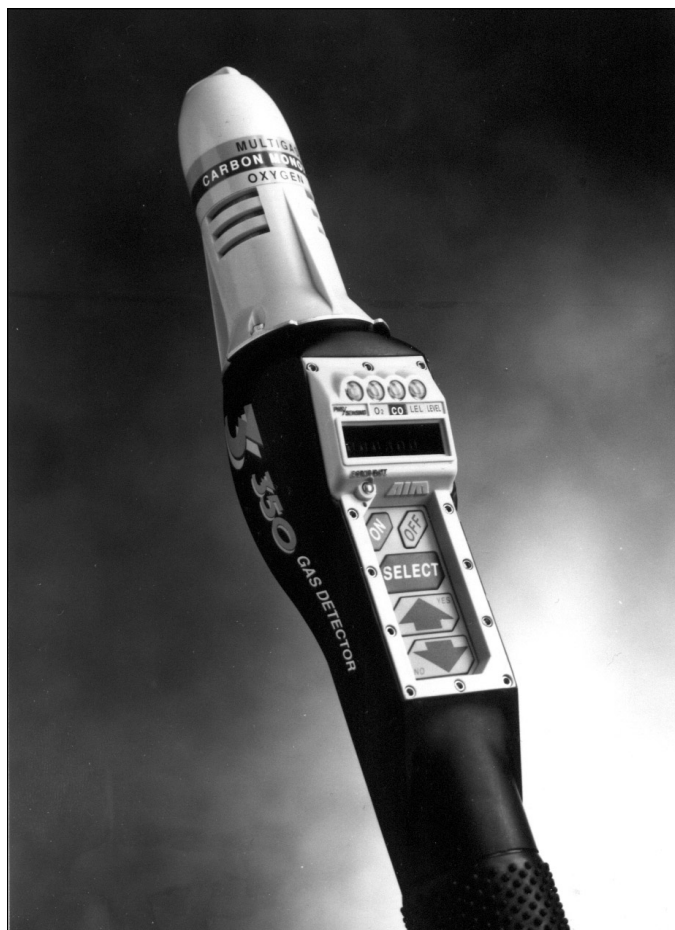
Figure 17–12. A multigas monitor using a metal oxide semiconductor sensor for combustible gases and electrochemical sensors for oxygen and toxic gases. (Courtesy AIM Safety USA, Inc.)
