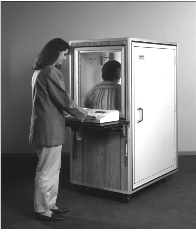
Figure 9-27. Sound booth audiometric testing. (Courtesy Tretmetrics Occupational Health Group.)
