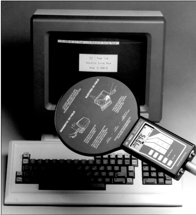
Figure 11-17. A displacement sensor is oriented so that its flat surface faces the source. (Courtesy Holaday Industries, Inc.)
