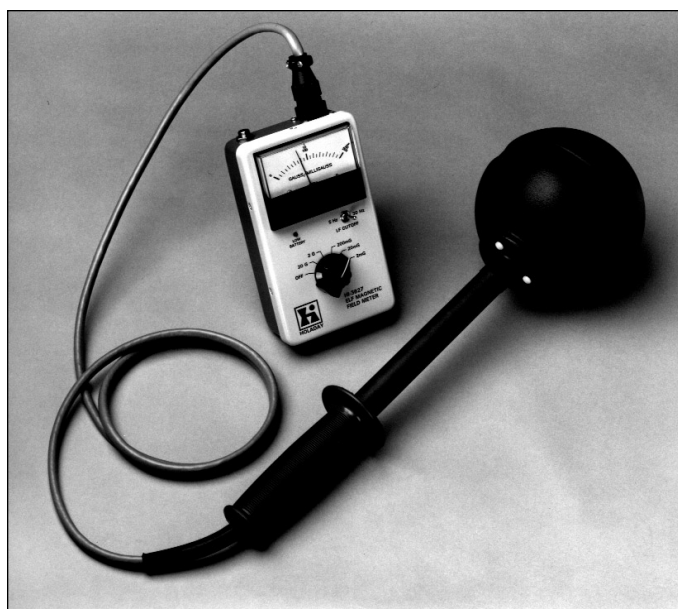
Figure 11-9. Loops are often ganged together in mutually orthogonal arrays of three loops. (Courtesy Holaday Industries, Inc.)
