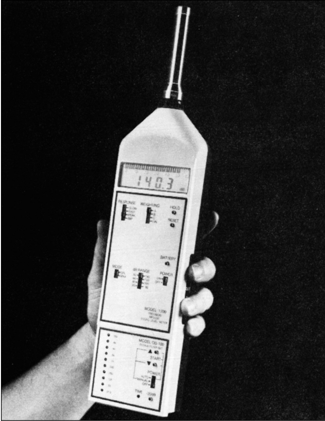
Figure 9-10. The multipurpose instrument shown here can be used as a sound level meter, octave-band analyzer, and impact/impulse noise meter. (Courtesy Quest Technologies.)
