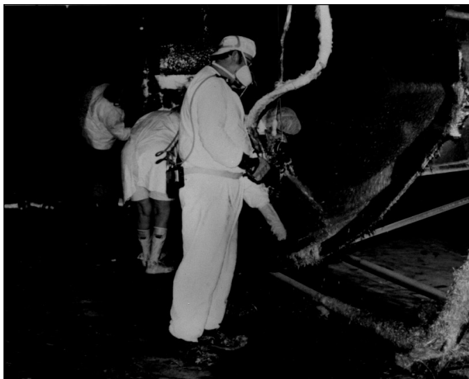
Figure 22-16. Workers wearing combination chemical cartridge/N95 particulate filter respirator for protection from solvent vapors and mists and glass fibers in a fiberglass operation. (Courtesy 3M.)
