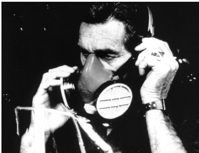
Figure 22-33. The isoamyl acetate qualitative fit test protocol requires respirators to be equipped with cartridges capable of removing organic vapors and uses a test enclosure. (Courtesy Survivair.)
