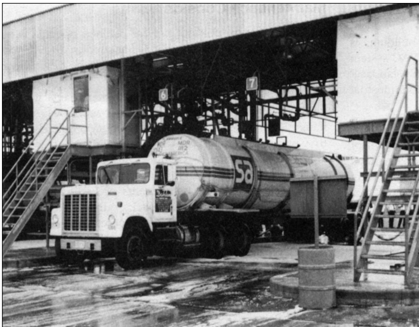
Figure 18-4. Loading or unloading of tank trucks can release airborne contaminants.
