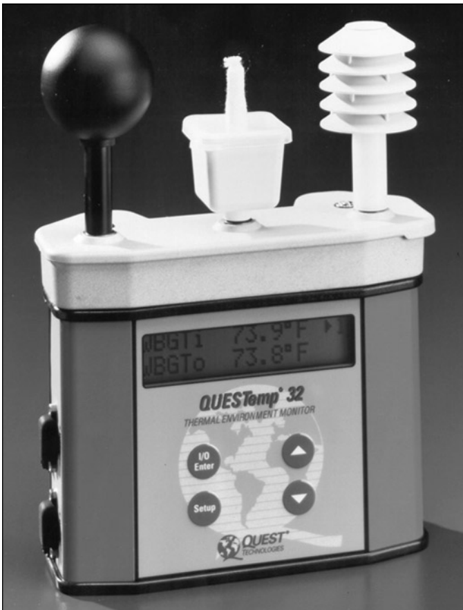
Figure 12–4. Examples of electronic devices used to measure WBGT. (Courtesy of Metrosonics, Inc., Quest Technologies, and IST.)
