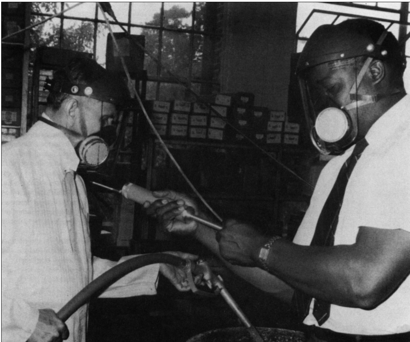
Figure 15-7. The gas detector tubes shown here are useful for obtaining direct readings of gas or vapor contamination in the workplace air.
