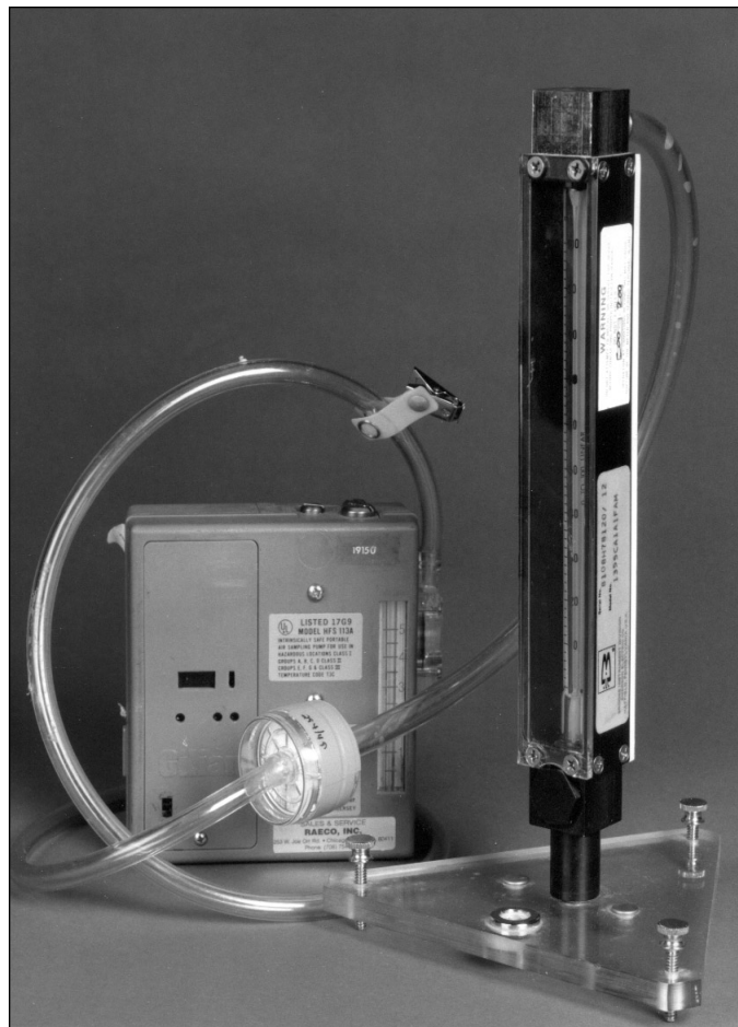
Figure 16–21. Precision rotameter connected to a sampling train. (Courtesy Fermilab Media Services Dept.)
