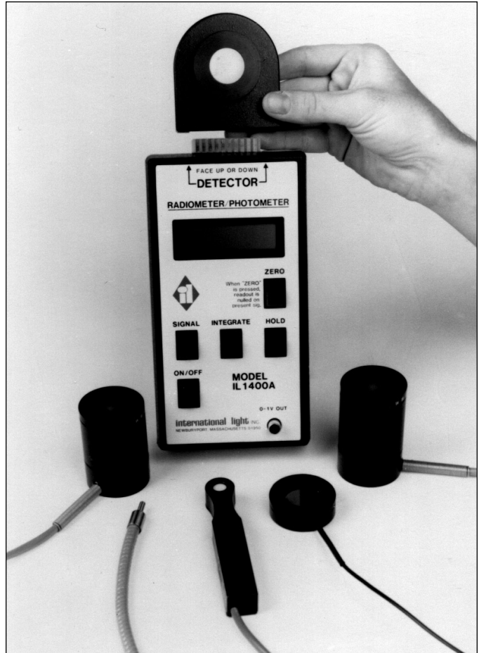
Figure 11–21. Instruments are now on the market that have wavelength response characteristics that approximate the spectral effectiveness curves of the TLVs. (Courtesy International Light, Inc.)
