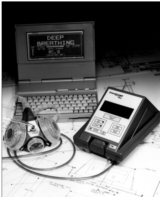
Figure 22-38. The ambient aerosol quantitative fit-test system does not use a test enclosure and must be used with respirators equipped with high efficiency filters. (Courtesy TSI.)
