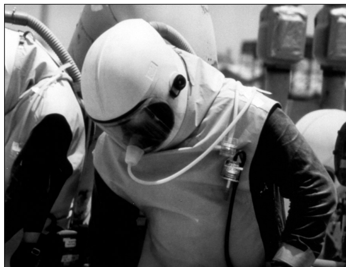
Figure 22–32. Workplace studies simultaneously measuring air contaminants outside and inside the respirator are being used to establish assigned protection factors for the classes of respirators. (Courtesy 3M.)
