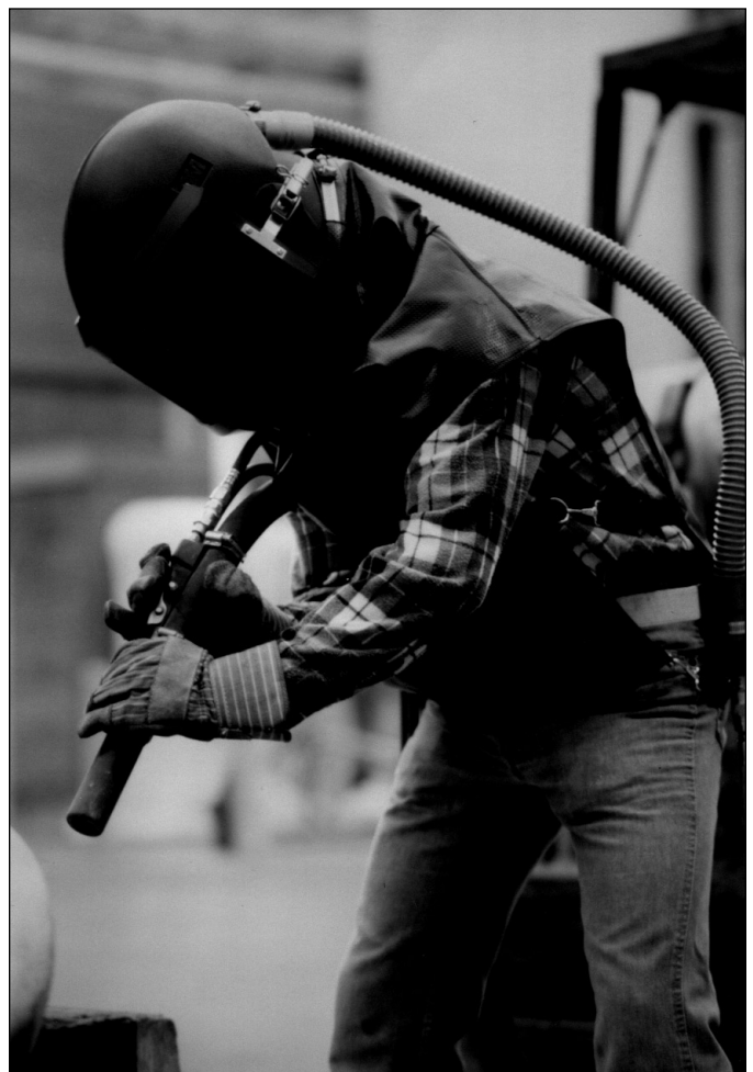
Figure 22–23. Abrasive blasting continuous flow air-line respirator. (Courtesy 3M.)
