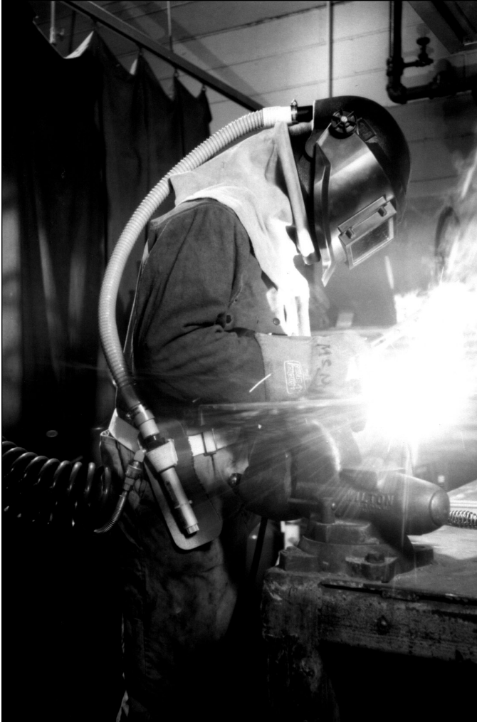
Figure 22–22. A continuous flow air-line respirator with a helmet with a viewing lens adapter for welding. (Courtesy 3M.)
