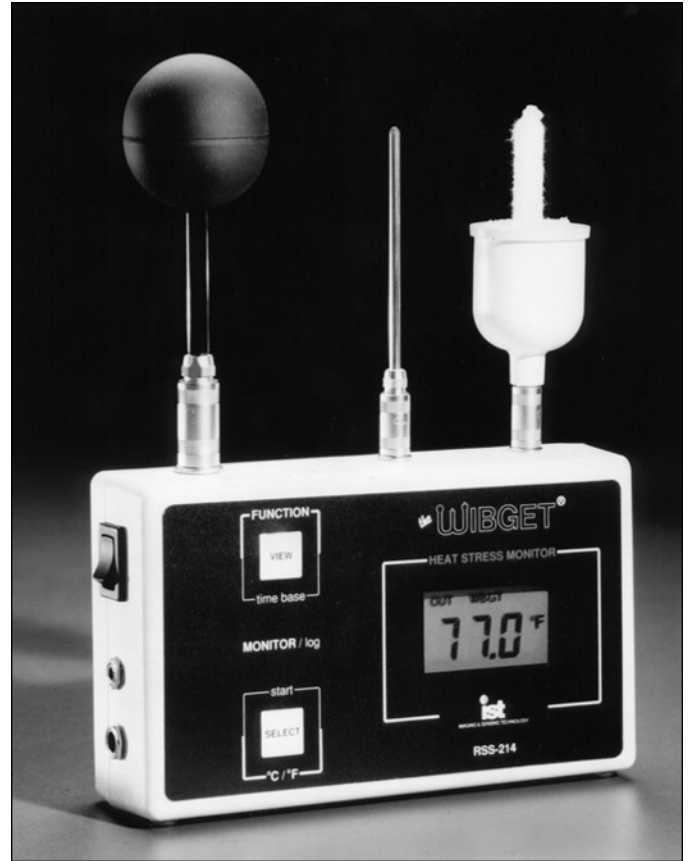
Figure 12–4. Examples of electronic devices used to measure WBGT. (Courtesy of Metrosonics, Inc., Quest Technologies, and IST.)
