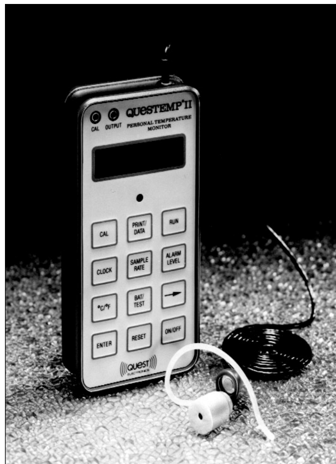
Figure 12–10. Photographs of two commercially available personal monitors developed for heat-stress exposures. (Courtesy of Metrosonics, Inc, and Quest Technologies.)
