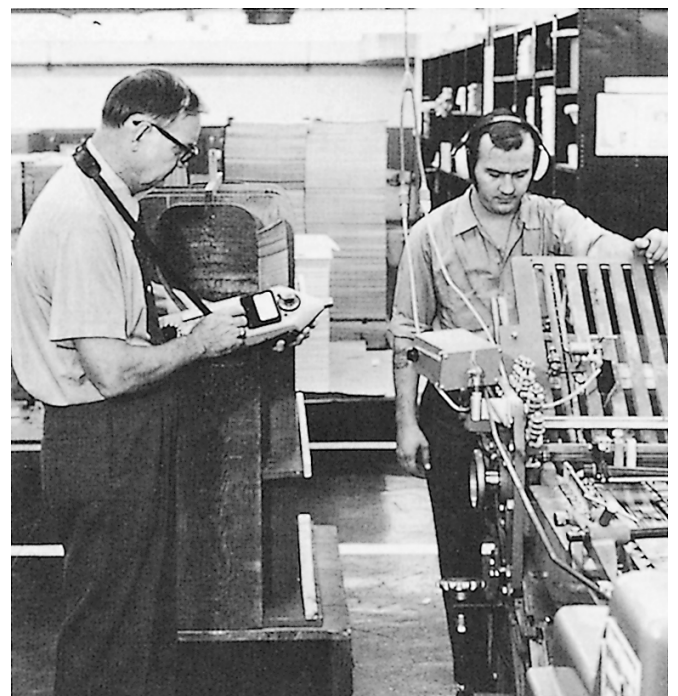
Figure 9-16. Take sound level measurements near an employee's workstation.
