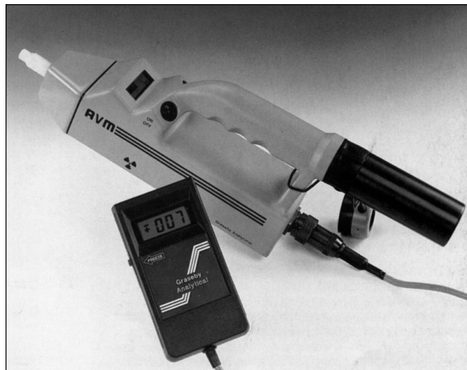
Figure 17-26. A portable TDI monitor based on the principles of ion mobility spectrometry. (Courtesy Graesby Environmental, Atlanta, Ga.)
