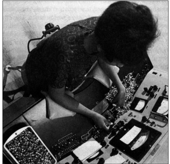
Figure 1–4. Worker uses pads to keep her forearm off the sharp table edge.
