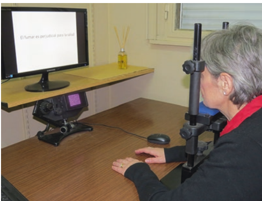
Fig. 21.1 Eye-movement registering process. The monitor can be seen, where the sentences are displayed, and the eye tracker (above the monitor), which consists of a 1,000 frames per second video camera and an infrared illuminator to increase pupil contrast and facilitate its detection
