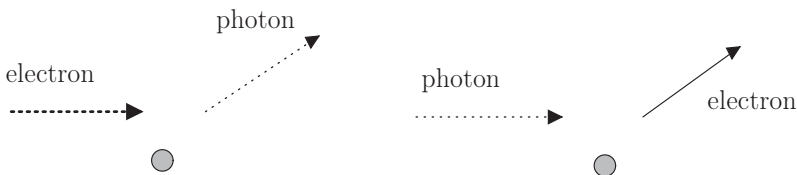
Fig. 2.18 Radiative recombination (left) and photoemission (right)
