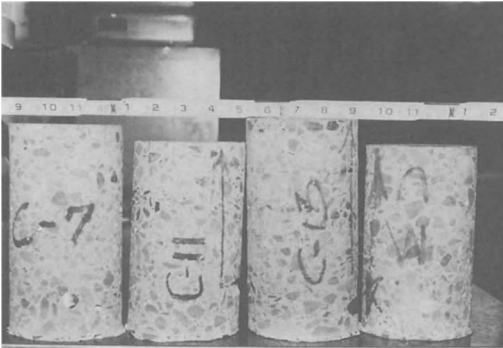
Figure 15-52. Several concrete core samples are obtained from selected locations for laboratory examination and testing.
