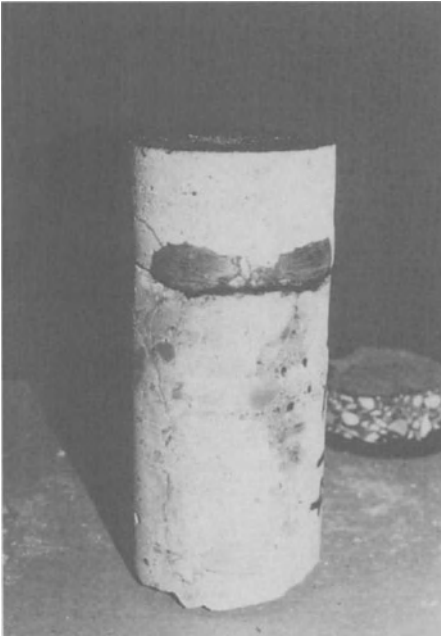
Figure 15-51. Core sample over previously patched areas with a waterproofing membrane and asphalt wearing surface.
