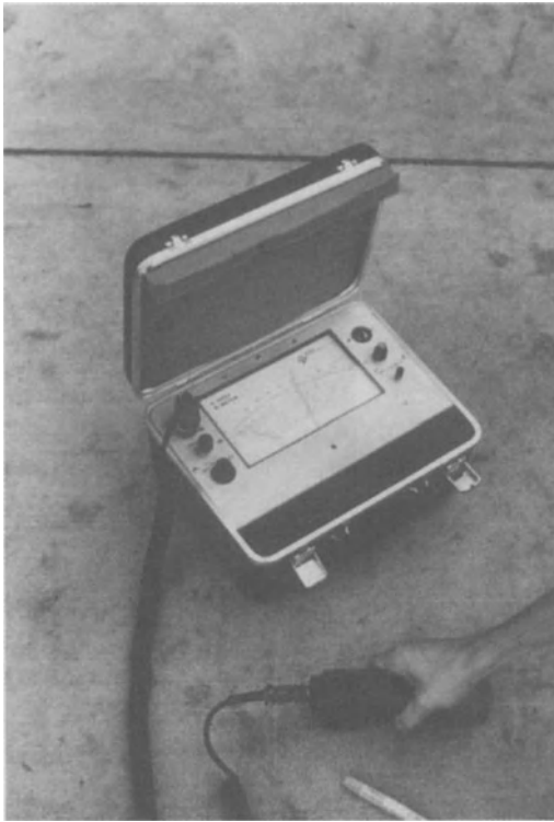
Figure 15-46. A pachometer is used to locate and measure concrete cover over embedded reinforcement.
