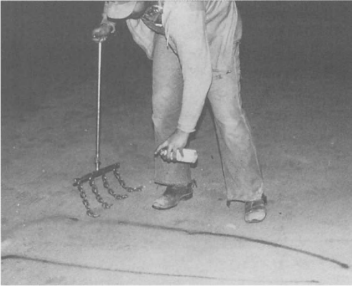
Figure 15-44. Boundaries of delaminated areas marked by spray chalk.
