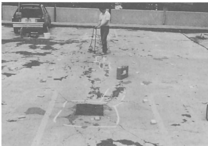
Figure 15-53. Half-cell potential measurement in field.
