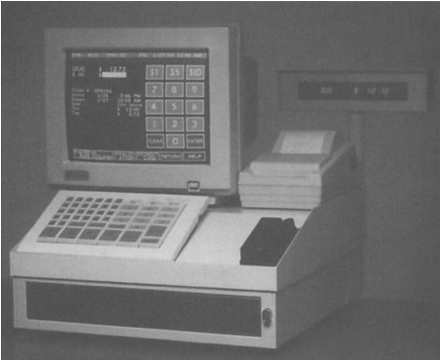
Figure 3-4. The fee computer provides an audit trail for control of cash revenues. Photo courtesy Parking Automation Corporation.
