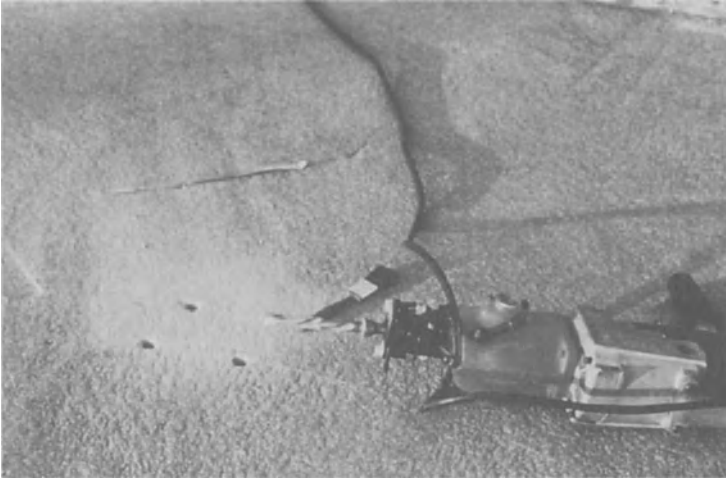
Figure 15-47. Obtaining concrete powder sample in field.
