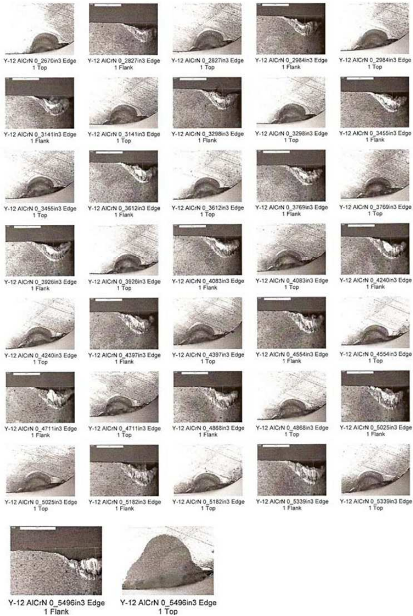
Figure 7.6. AlCrN Tool Cutting Edge 1 machined at 121 RPM. 0.2670 - 0.5496 in 3 workpiece removed
