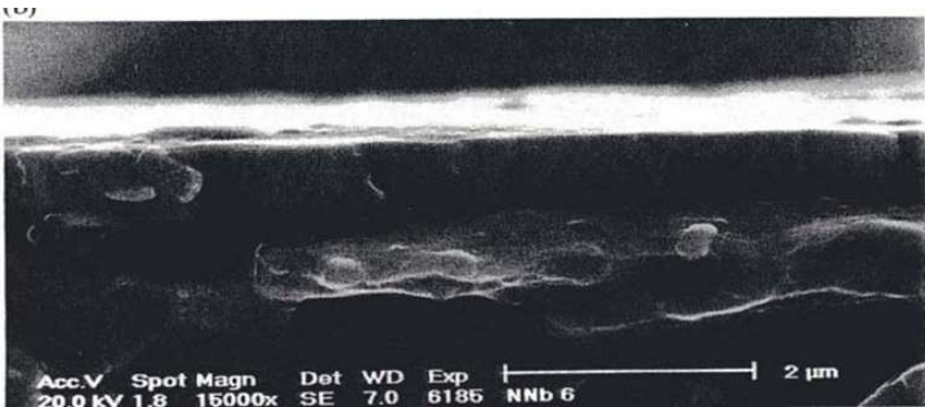
Figure 4.36. Coatings Deposited at -125\text{V} Bias [71]
