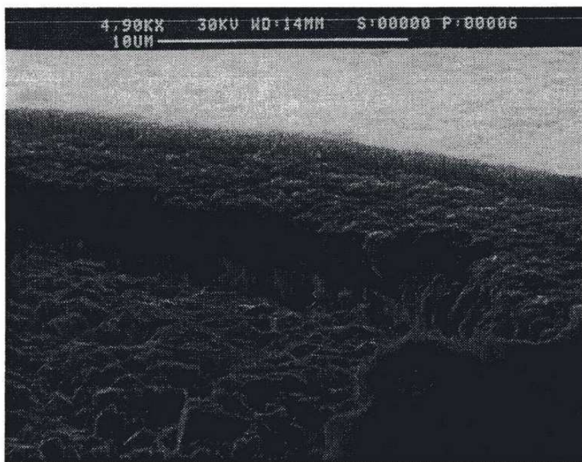
Figure 4.17. Fracture of the Coating [52]
