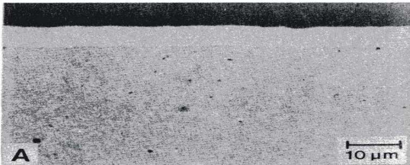
Figure 4.25. PVD Deposited TiN on Alloy A [58]
