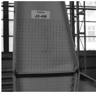
Figure 5b. Failure mode of specimen J2-4m – monotonic loading
