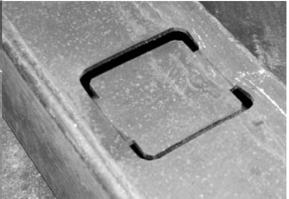
Figure 7: View of chord face failure WTL2 Figure 8: View of chord face failure WTL2
