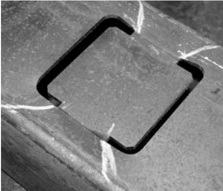
Figure 7: View of chord face failure WTL2 Figure 8: View of chord face failure WTL2
