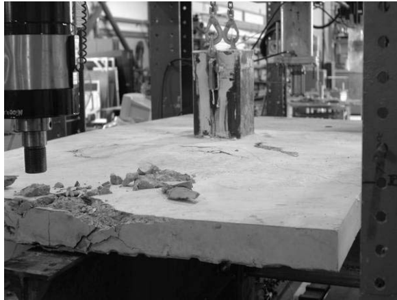
Figure 7: Shear connectors pull out and concrete failure.
