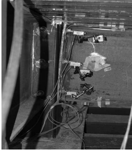
Figure 6: Blind bolts of the endplate displace 3 mm outwards.
