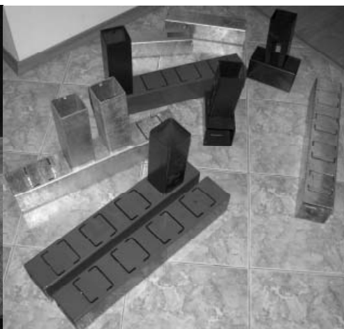
Figure 2: Laser cut of chord and branch locks & elements
