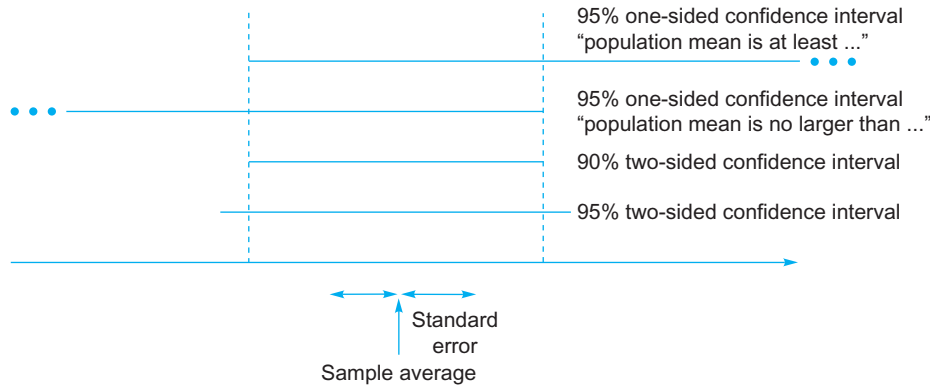
FIG. 9.4.1 Both kinds of one-sided confidence intervals are illustrated at the top. One-sided confidence intervals always include the sample average, starting from a point on one side and continuing indefinitely on the other. Note that the endpoint for the 95% one-sided confidence interval is the same as one of the endpoints for the 90% two-sided confidence interval.
