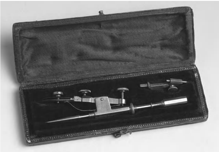
Fig. 6.47 Compass to draw circles of very small radius
