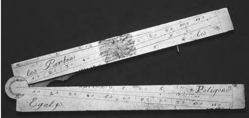
Fig. 2.12 Realization of Butterfield, an engineer of Louis XIV. The represented object is a geometric compass, made with fine workmanship, brass, engraved with figures, is signed by Butterfield and carries the words “Paris Cordes, les Métaux;” “the Parties Egales” and “Polygons” (Brunetti and Rovida 2006)
