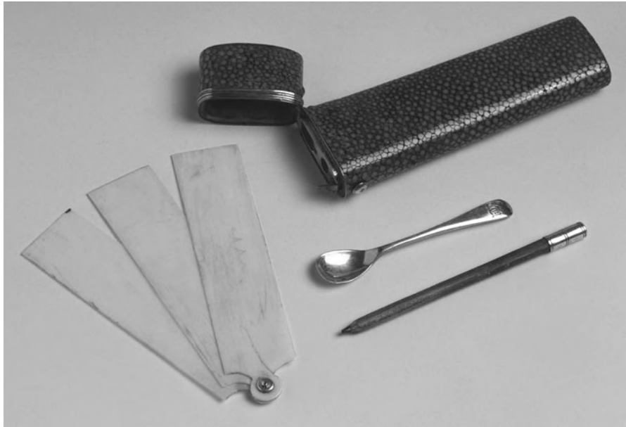
Fig. 5.52 Complex of drawing instruments, signed Jo. Anningson, constituted by a spoon, a pencil and a block notes, consisting of thin sheets of ivory (Brunetti and Rovida 2006)
