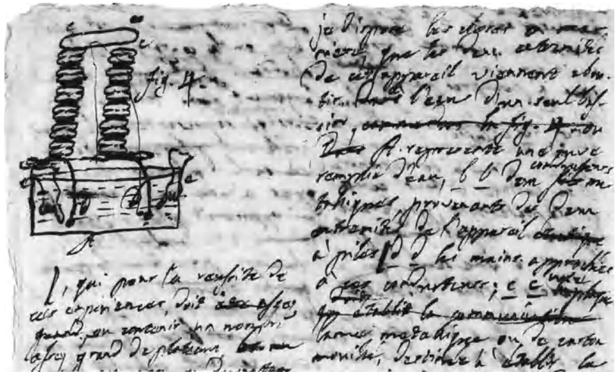
Fig. 5.35 Representation of the Voltaic pile: interesting is the section lining, to represent the “section” of the liquid
