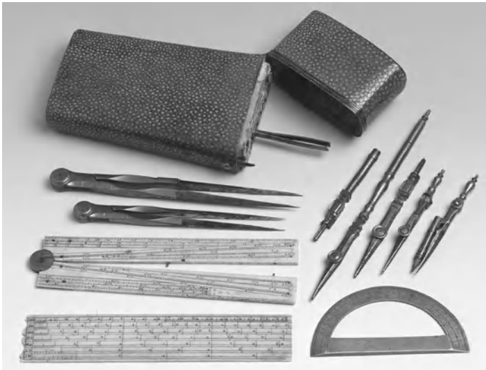
Fig. 6.49 Drawing complete that contains 11 pieces, among them, drawing pens, compasses, ruler and geometric compass. The case is covered with fish skin (a very common feature in the Nineteenth Century)
