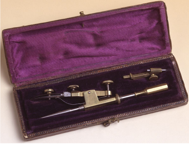
Fig. 7.59 Compass to draw circles with very small radius (principle of the Twentieth Century)
