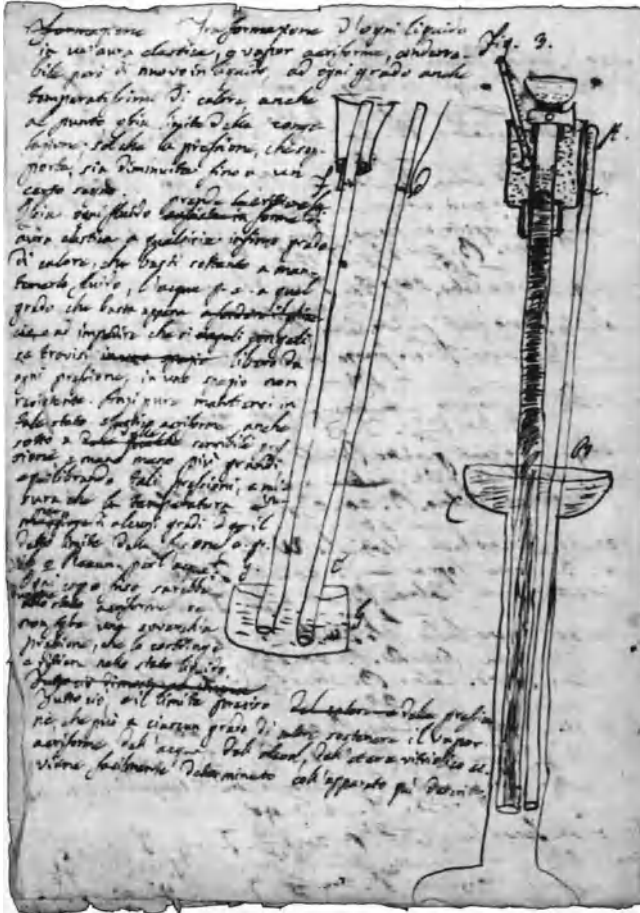
Fig. 5.39 Another representation of an experiment: interesting is the section lining to represent the “section” of liquid and of gas
