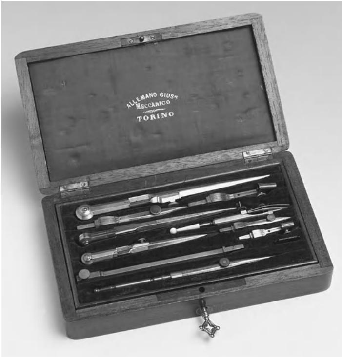
Fig. 6.48 Italian compasses of the nineteenth century. The case is realized with high accuracy and elegance
