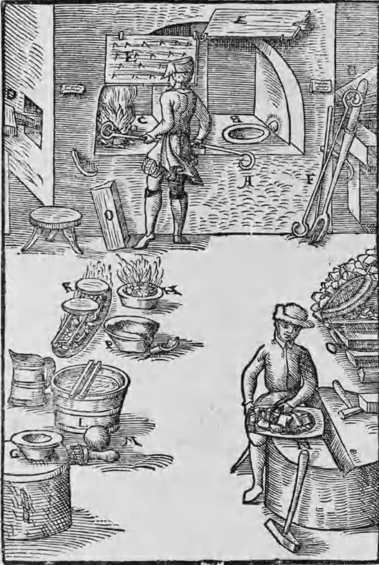
Fig. 4.28 Workshop for silver refining by Lazarus Eckert (end of the sixteenth century)
