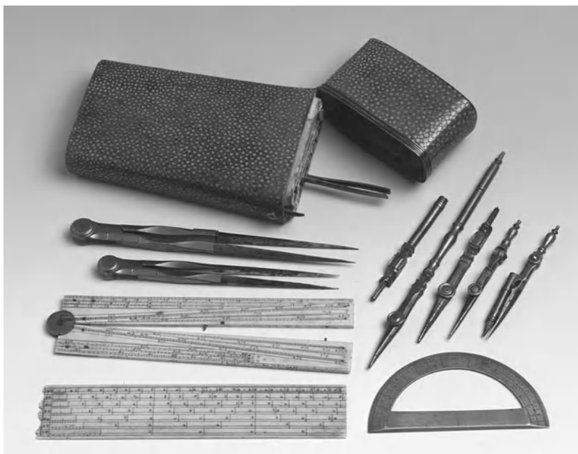
Fig. 2.11 Drawing instruments (eighteenth century) (11 pieces, among them, drawing pens, compasses, ruler and geometric compass. The case is covered with fish skin, a very common feature in the nineteenth century) (Brunetti and Rovida 2006)
