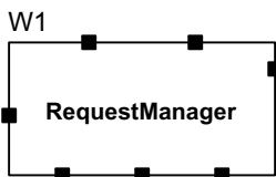
Figure 7-14. An object with pins
