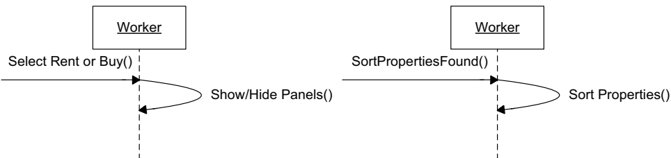
Figure 10-6. User actions that the Worker can handle by itself
