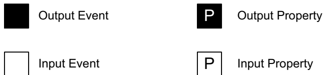
Figure 6-28. Port symbols used in later versions of Connector diagrams
