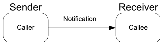
Figure 3-16. A notification delivered using a procedure call
