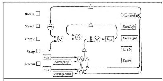
**Figure 7.21** The circuit for determining whether the agent is at [1,1]. Every location and orientation register has a similar circuit attached.
