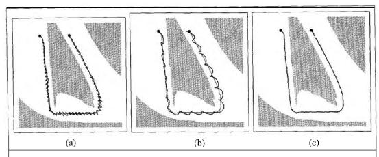
**Figure 25.20** Robot arm control using (a) proportional control with gain factor 1.0, (b) proportional control with gain factor 0.1, and (c) PD control with gain factors 0.3 for the proportional and 0.8 for the differential component. In all cases the robot arm tries to follow the path shown in gray.
