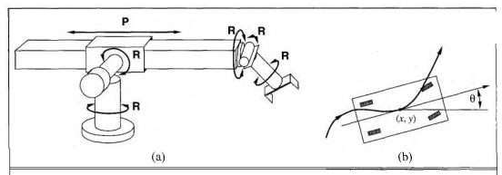
**Figure 25.3** (a) The Stanford Manipulator, an early robot arm with five revolute joints (R) and one prismatic joint (P), for a total of six degrees of freedom. (b) Motion of a nonholonomic four-wheeled vehicle with front-wheel steering.
