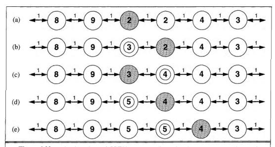
**Figure 4.22** Five iterations of  $LRTA^*$  on a one-dimensional state space. Each state is labeled with H(s), the current cost estimate to reach a goal, and each arc is labeled with its step cost. The shaded state marks the location of the agent, and the updated values at each iteration are circled.
