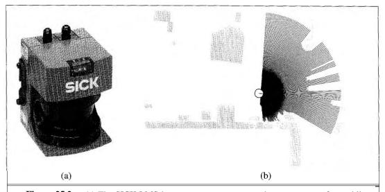
**Figure 25.2** (a) The SICK LMS laser range scanner; a popular range sensor for mobile robots. (b) Range scan obtained with a horizontally mounted sensor, projected onto a two-dimensional environment map.
