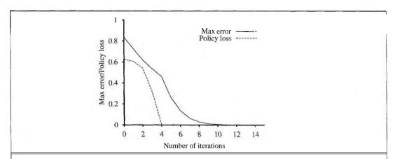
**Figure 17.6** The maximum error  $||U_i - U||$  of the utility estimates and the policy loss  $||U^{\pi_i} - U||$  compared with the optimal policy, as a function of the number of iterations of value iteration.
