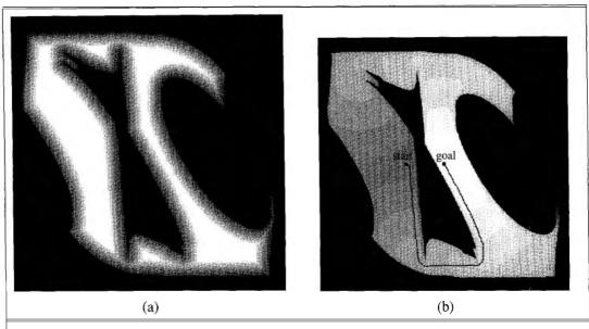
**Figure 25.15** (a) A repelling potential field pushes the robot away from obstacles. (b) Path found by simultaneously minimizing path length arid the potential.
