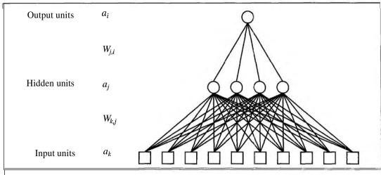
**Figure 20.24** A multilayer neural network with one hidden layer and 10 inputs, suitable for the restaurant problem.
