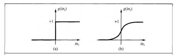
**Figure 20.16** (a) The **threshold** activation function, which outputs 1 when the input is positive and 0 otherwise. (Sometimes the **sign** function is used instead, which outputs  $\pm 1$  depending on the sign of the input.) (b) The **sigmoid** function  $1/(1 + e^{-x})$ .
