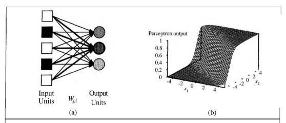
**Figure 20.19** (a) A perceptron network consisting of three perceptron output units that share five inputs. Looking at a particular output unit (say the second one, outlined in bold), we see that the weights on its incoming links have no effect on the other output units. (b) A graph of the output of a two-input perceptron unit with a sigmoid activation function.
