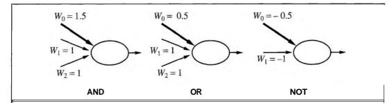
**Figure 20.17** Units with a threshold activation function can act as logic gates, given appropriate input and bias weights.
