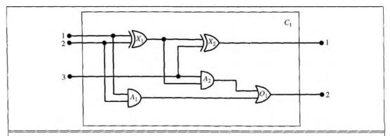
**Figure 8.4** A digital circuit C1, purporting to be a one-bit full adder. The first two inputs are the two bits to be added and the third input is a carry bit. The first output is the sum, and the second output is a carry bit for the next adder. The circuit contains two XOR gates, two AND gates and one OR gate.
