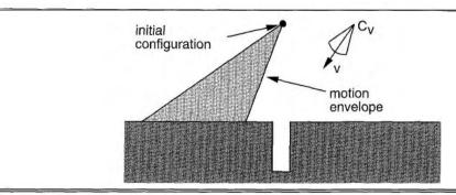
**Figure 25.18** The first motion command and the resulting envelope of possible robot motions. No matter what the error, we know the final configuration will be to the left of the hole.
