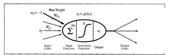
**Figure 20.15** A simple mathematical model for a neuron. The unit's output activation is  $a_i = g(\sum_{j=0}^n W_{j,i}a_j)$ , where  $a_i$  is the output activation of unit j and  $W_{j,i}$  is the weight on the link from unit j to this unit.
