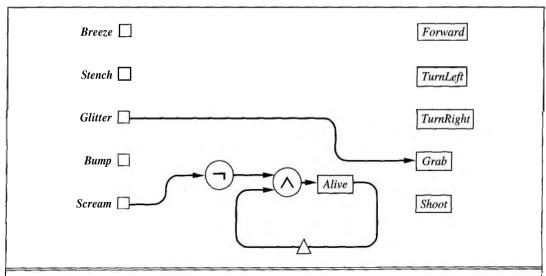
**Figure 7.20** Part of a circuit-based agent for the wumpus world, showing inputs, outputs, the circuit for grabbing the gold, and the circuit for determining whether the wumpus is alive. Registers are shown as rectangles and one-step delays are shown as small triangles.
