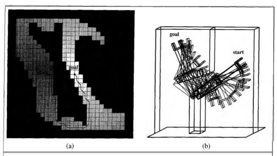
**Figure 25.14** (a) Value function and path found for a discrete grid cell approximation of the configuration space. (b) The same path visualized in workspace coordinates. Notice how the robot bends its elbow to avoid a collision with the vertical obstacle.
