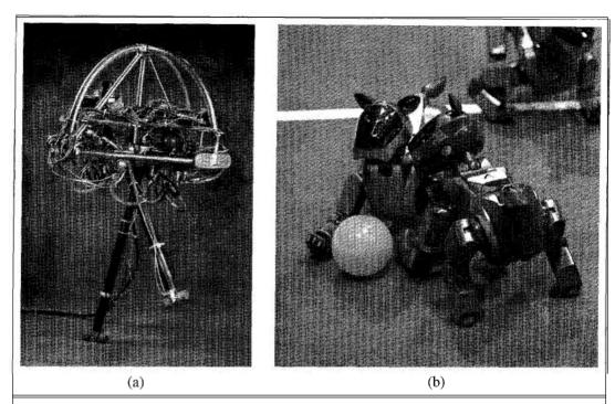
**Figure 25.4** (a) One of Marc Raibert's legged robots in motion. (b) Sony AIBO robots playing soccer. (© 2001, The RoboCup Federation.)
