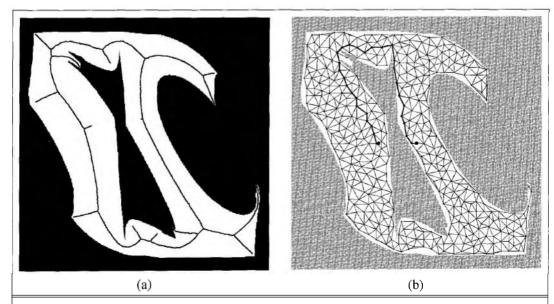
**Figure 25.16** (a) The Voronoi diagram is the set of points equidistant to two or more obstacles in configuration space. (b) A probabilistic roadmap, composed of 400 randomly chosen points in free space.
