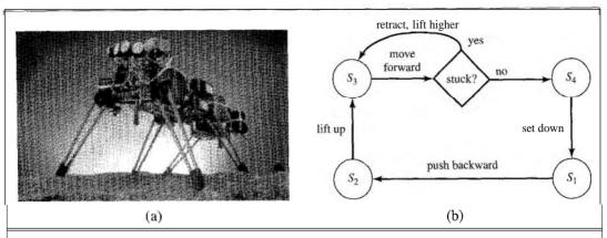
**Figure 25.22** (a) A hexapod robot (b) An augmented finite state machine (AFSM) for the control of a single leg. Notice that this AFSM reacts to sensor feedback: if a leg is stuck during the forward swinging phase, it will be lifted increasingly higher.
