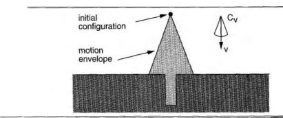
**Figure 25.17** A two-dimensional environment, velocity uncertainty cone, and envelope of possible robot motions. The intended velocity is v, but with uncertainty the actual velocity could be anywhere in  $C_v$ , resulting in a final configuration somewhere in the motion envelope, which means we wouldn't know if we hit the hole or not.
