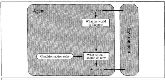
**Figure 2.9** Schematic diagram of a simple reflex agent.
