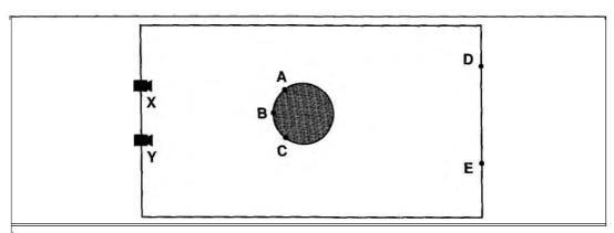
**Figure 24.25** Top view of a two-camera vision system observing a bottle with a wall behind.
