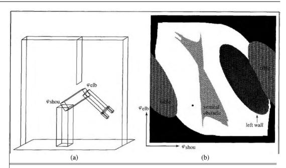
**Figure 25.12** (a) Workspace representation of a robot arm with 2 DOFs. The workspace is a box with a flat obstacle hanging from the ceiling. (b) Configuration space of the same robot. Only white regions in the space are configurations that are free of collisions. The dot in this diagram corresponds to the configuration of the robot shown on the left.
