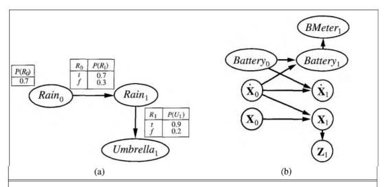
**Figure 15.11** (a) Specification of the prior, transition model, and sensor model for the umbrella DBN. All subsequent slices are assumed to be copies of slice 1. (b) A simple DBN for robot motion in the X–Y plane.
