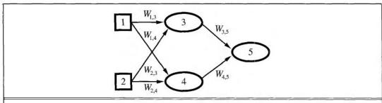
**Figure 20.18** A very simple neural network with two inputs, one hidden layer of two units, and one output.
