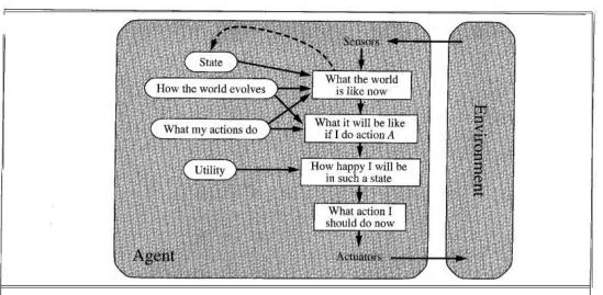
**Figure 2.14** A model-based, utility-based agent. It uses a model of the world, along with a utility function that measures its preferences among states of the world. Then it chooses the action that leads to the best expected utility, where expected utility is computed by averaging over all possible outcome states, weighted by the probability of the outcome.
