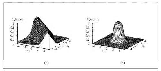
**Figure 20.23** (a) The result of combining two opposite-facing soft threshold functions to produce a ridge. (b) The result of combining two ridges to produce a bump.
