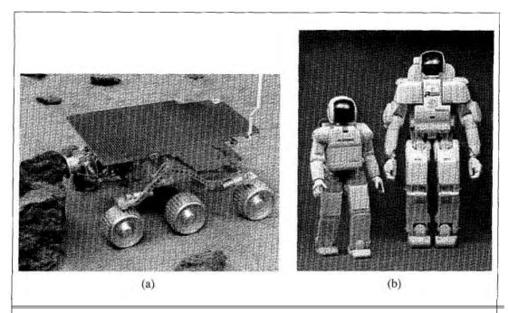
**Figure 25.1** (a) NASA's Sojourner, a mobile robot that explored the surface of Mars in July 1997. (b) Honda's P3 and Asimo humanoid robots.
