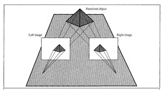
**Figure 24.10** The idea of stereopsis: different camera positions result in slightly different two-dimensional views of the same three-dimensional scene.
