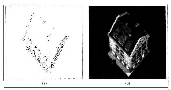
**Figure 24.9** (a) three-dimensional reconstruction of the locations of the image features in Figure 24.8, shown from above. (b) The real house, taken from the same position.
