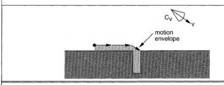
**Figure 25.19** The second motion command and the envelope of possible motions. Even with error, we will eventually get into the hole.
