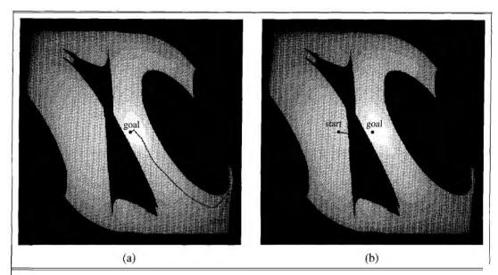
**Figure 25.21** Potential field control. The robot ascends a potential field composed of repelling forces asserted from the obstacles, and an attracting force that corresponds to the target configuration. (a) Successful path. (b) Local optimum.
